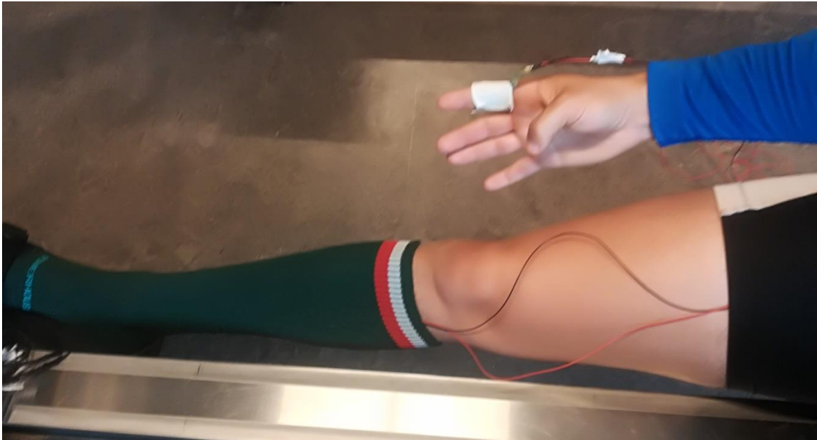
FIGURE 30 SENSORS PLACED IN SOCK AND AT THE HANDS
