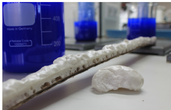
Figure 50: The spray foam
