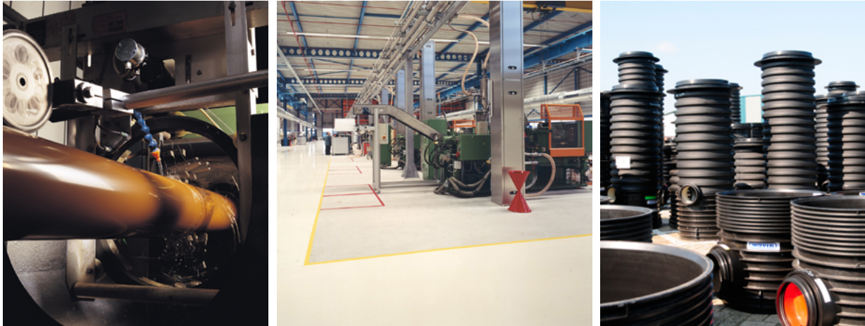
Figure 1: The extrusion process of PVC pipes (left), the injection molding factory (middle) and the Tegra range (right), derived from Wavin Brand Portal.
