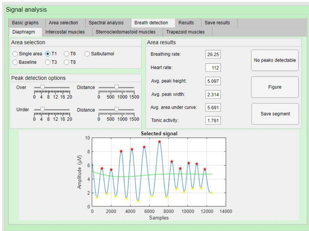
**Figure 34:** Overview of the breath detection pane. The user is required to select a muscle group pane and a timeframe. The application then automatically calculates the parameters found on the righthand side. The user may alter the detection thresholds if the standard algorithm does not suffice.
