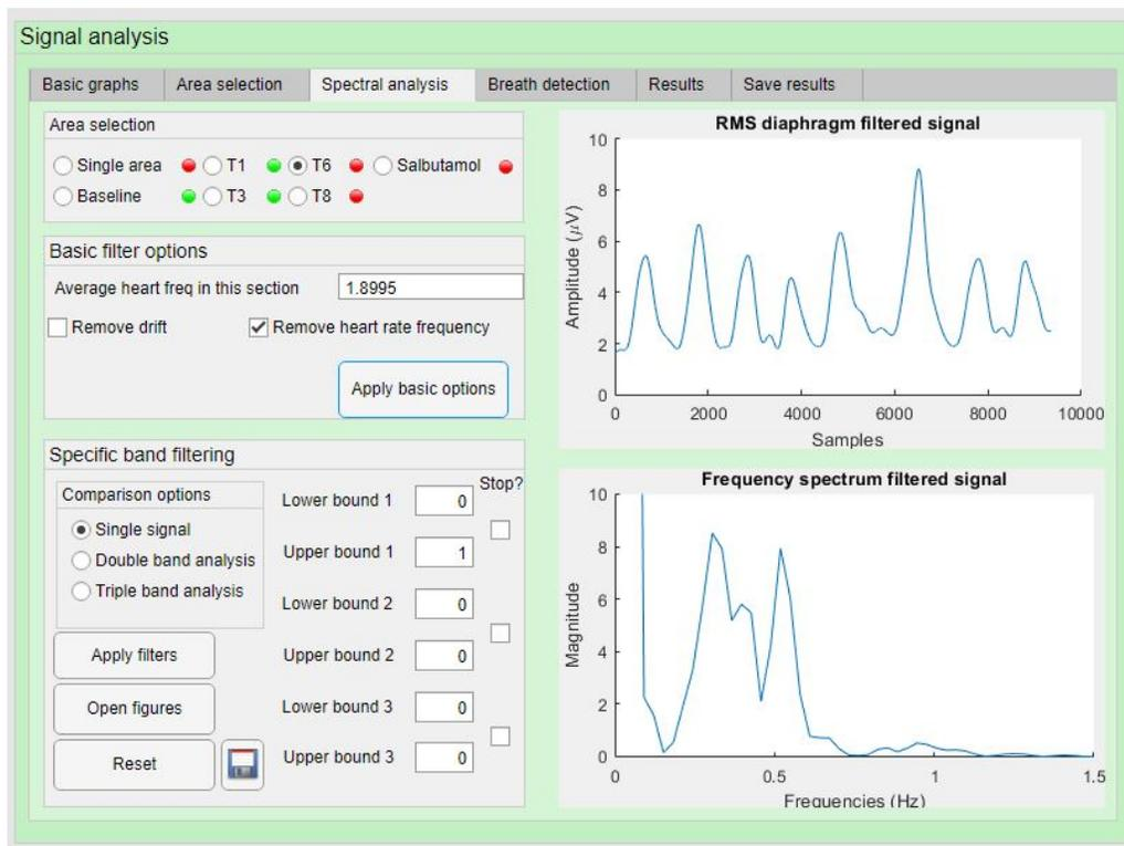
**Figure 33:** Overview of the spectral analysis pane. The user is presented with various filtering options to remove any artefact frequencies from the signal.
