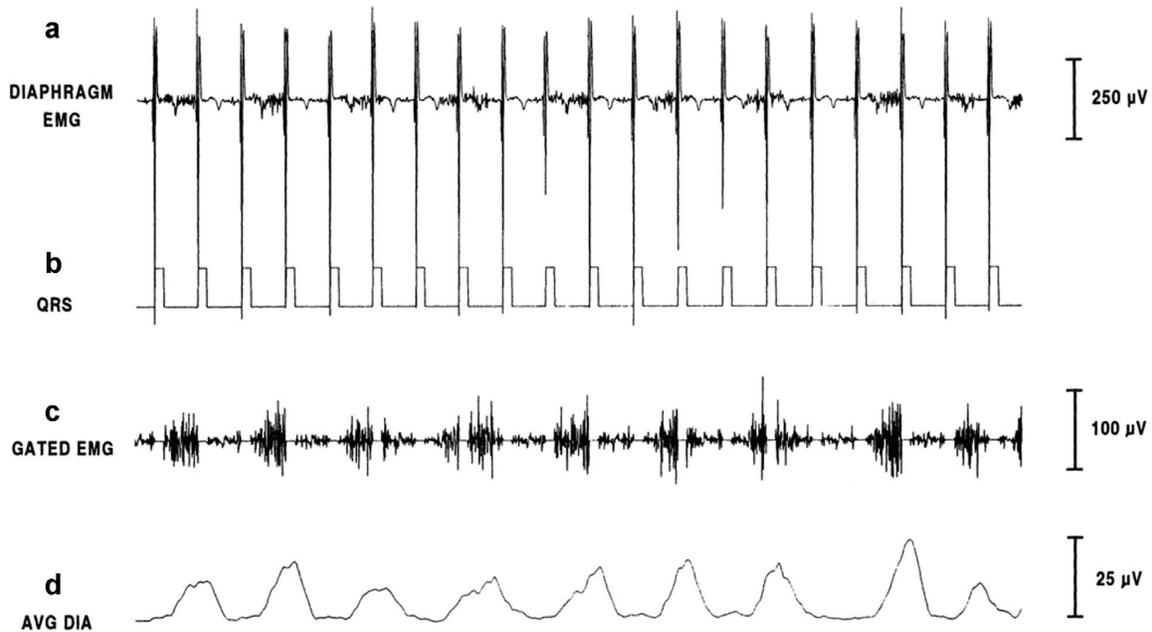
**Figure 9:** Overview of the different stages of signal processing using the gating technique. a) The raw measured data, containing clear large QRS complexes. b) Detection of QRS complex as a standard pulse with the width of the QRS complex. c) Gated EMG signal, the QRS complex is replaced with a running average at the length of the QRS complex. d) Averaged EMG signal by computing the RMS of the gated EMG signal, the signal used for analysis. (Adapted from O’Brien et al. [24])
