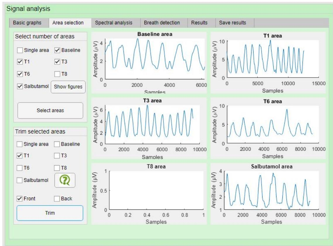
**Figure 32:** Area selection panel. The user is required to select the timeframes applicable to the measured patient, corresponding with the amount of spirometry measurements performed.
