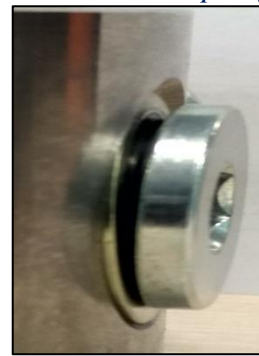
Figure. E-12: BS ring guided by the chamfer and the ring is being centered around the neck of the plug.
