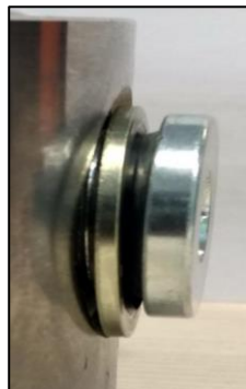
Figure. E-11: BS ring outer edge in contact with the chamfered edge of the hole.
