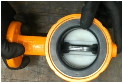
Figure. A-3: Aligning the body over the disc using the center line as a reference (Figure. A-2) to attain an accurate alignment of shaft holes.
