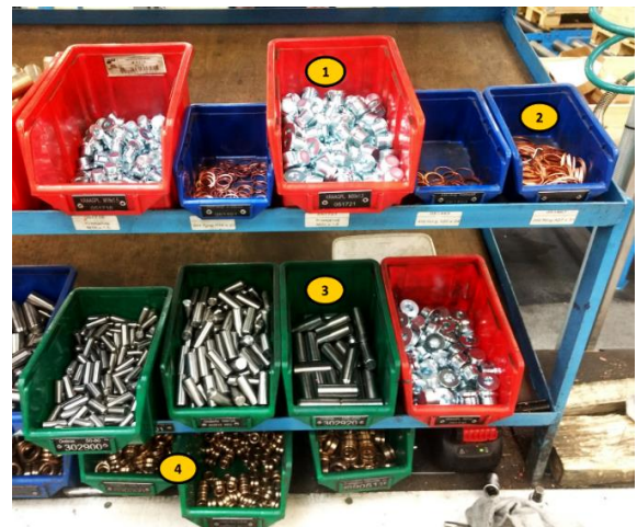
Figure 1-6: Uniquely identified kanban bins for all the plugs (1), sealing rings (2), bottom shafts (3), and o-ring bushing (4). The black strips on the bins have a unique article number, used for identification of components as per production order.
