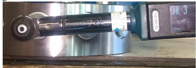
Figure 3-18: Tightening the plug & ring in the test ring at 10 Nm torque.
