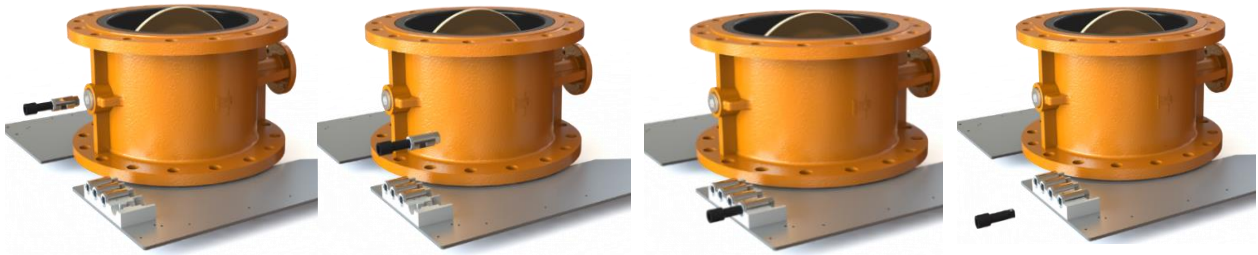
Figure 5-12: The system retracts & follows the prior steps in reverse order to place the tool bit back inside the fixture and go back to its home position
