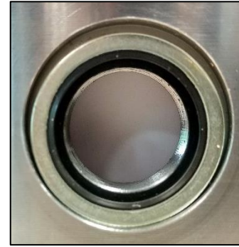
Figure. E-9: ScBS ring inside the counterbore hole with larger clearance around the circumference. Though the Ring is eccentric, the inner centering projection of the ring covers the threaded hole and thus assures leak proofing.
