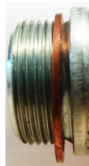
Figure 3-5: M36 Plug with sealing ring of copper in a non-concentric orientation about the plug.
