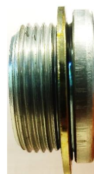
Figure 3-6: M36 plug with a bonded sealing ring with a non-concentric orientation about the plug.
