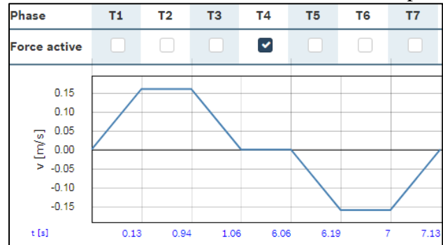
Figure 5-17: Velocity vs. time graph, showing the 7 different phases during translation. T1-T3 depicts forward stroke, T4 is the dwell phase, and finally, T5-T7 is the reverse stroke [33]
