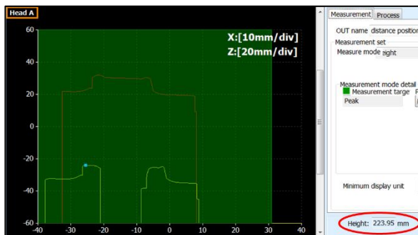
Figure 6-5: The yellow outline shows the position of the bottom hole of the body when compared with the standard outline of the body (determined at a fixed position as shown by the red colored profile). The straight line distance of the body from the sensor was determined to be 223.95mm.
