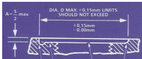
Figure. C-4: Spot face diameter for bonded seals [45]
