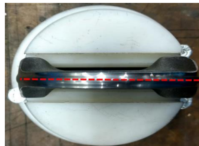
Figure. A-2: Disc accurately centered in the disc fixture and the red line denotes the center line of the disc, with a machined face as a reference edge.
