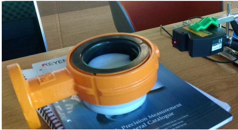
Figure 6-3: The test setup to determine the position of the bottom hole using the LVJ-2000 sensor.
