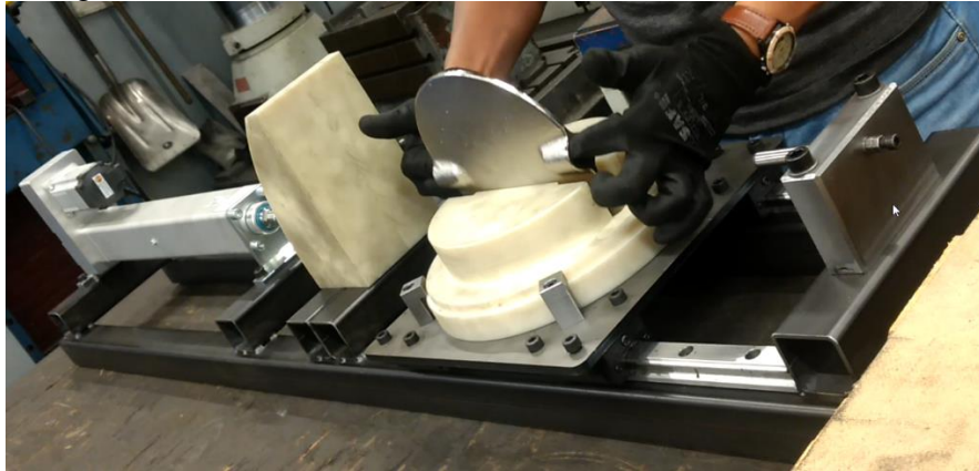
Figure. B-1: Placing the disc in the disc fixture with a hexagonal hole of the disc towards the force applicator cylinder.
