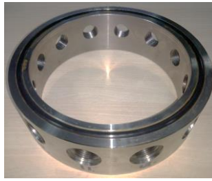
Figure. E-1: Leak test ring for plug size M27x2. Figure. E-2: The simulation results show the maximum stress of 3.185e^{+007} \text{ N/m}^2 and a maximum deformation of 6.126e^{-003} \text{ mm} .
