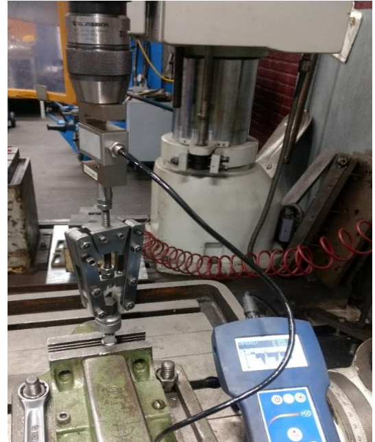
Figure. F-7: Test setup for determining the pull force required to detach a tool bit used for the M36 plug.
