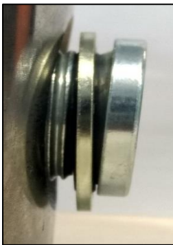
Figure. E-10: BS ring eccentric to the plug and hanging loose.
