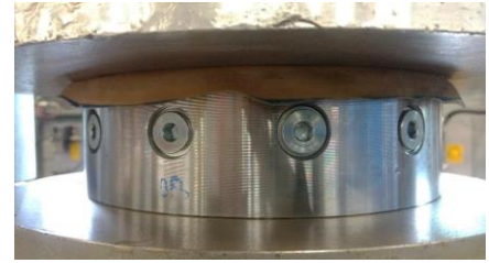
Figure. E-6: The press is closed, and the water is pressurized to 37.5 bar and left in this condition for 15min. After 15mins each plug is checked for visible leakage and results are noted.
