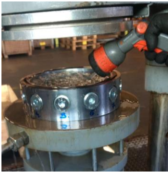
Figure. E-4: The completely assembled ring is kept on the leak test machine and filled with water up to its brim
