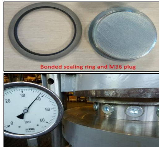
Figure 3-4: No leakage past the bonded sealing ring and plug when the plug is tightened with a torque of 50-Nm [39]
