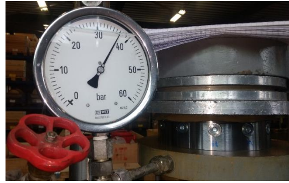
Figure 3-19: Testing the assembled ring at 37.5 bar pressure for 10mins to check for visible leakage.
