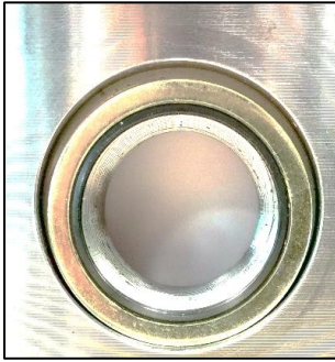
Figure. E-7: BS ring eccentric to the threaded hole and the lower edge of the vulcanized rubber does not cover the threaded hole. Thus, compromised sealing.
