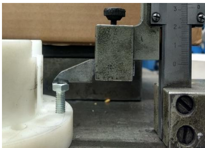
Figure. A-1: Adjusting the leveling screw to the desired height using a height gauge (in this case 23.9mm – half of the face to face thickness of an EVBS DN 80 valve)
