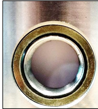
Figure. E-8: BS ring completely covers the threaded hole because of its close fit inside the counterbored hole.
