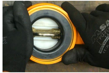
Figure. A-4: Body being pushed over the disc to assure the body rests against the height adjustment screws to eliminate misalignment errors.
