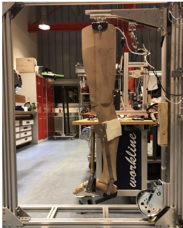
FIGURE 4.5: Illustration of the hanging leg experiment configuration.
