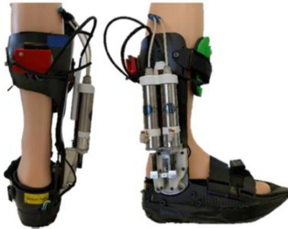
FIGURE 1.2: Back and side view of the PPAFO exoskeleton [10].
