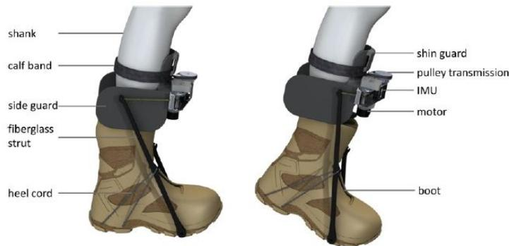
FIGURE 1.8: MIT Autonomous exoskeleton [14].
