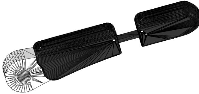
**Figure 4.8:** SolidWorks model of the ReFlex TakkTile used to derive inertial properties.
