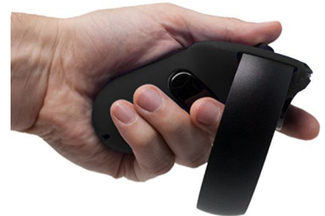
Fig.38: Grip button of the Oculus Touch controller, under the user's middle finger [xx].
