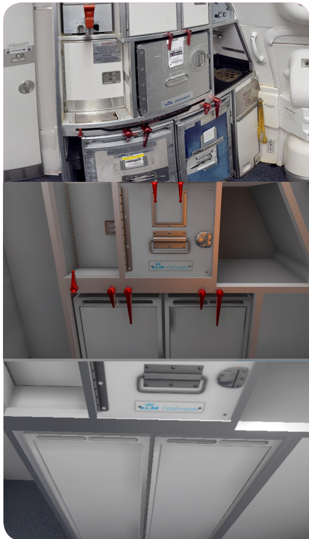
Fig.59: The locks guarding the trolleys were removed. Top: Real-life galley, middle: 1:1 virtual model, bottom: trolley locks removed
