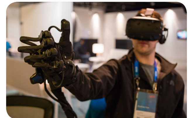
Fig. 14: HaptX gloves provide simulated haptic feedback [i]
