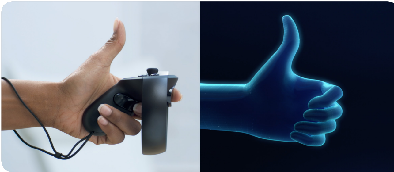
Fig.39: The Oculus Touch Controllers are able to approximate the stance of the user's hand [xxi]
