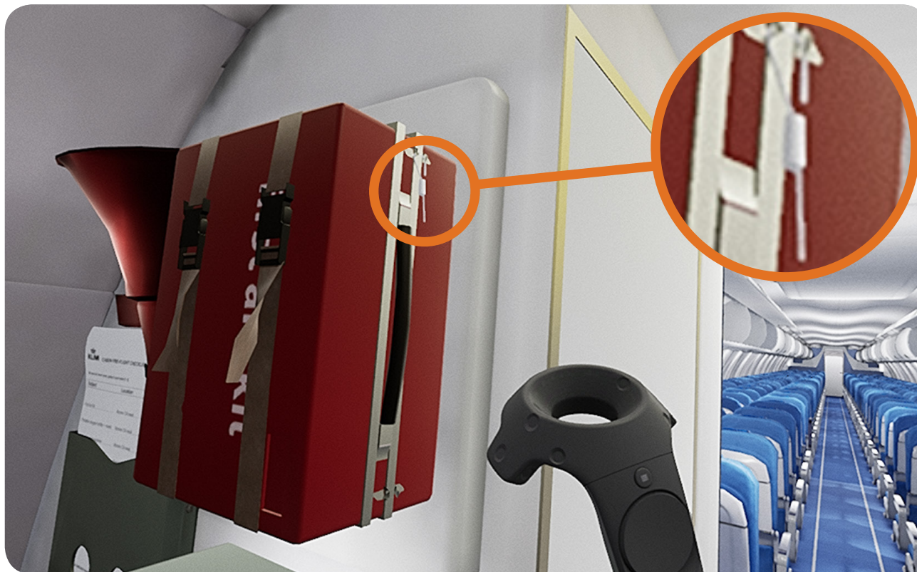
Fig.23: The seal of the first-aid kit (circled) in the pre-flight safety checklist VR-training. The screen door effect caused by limitations in the resolution of the VR headset makes it difficult to distinguish. A close up of the seal is shown on the right.
