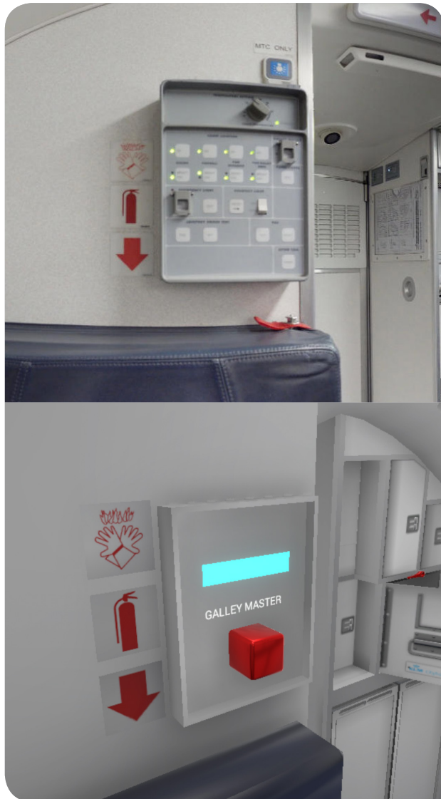
Fig. 54: Top: real-life crew control panel, bottom: the redesigned galley master button.
