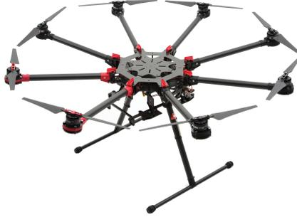
Figure 2.3: Example of an underactuated octo-rotor [5]
