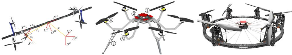
(a) Unusually shaped fully actuated hexarotor [8] (b) Fully actuated hexarotor [7] (c) FAST-Hex tiltable hexarotor [12]
