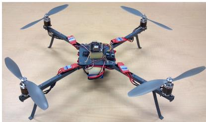
Figure 2.2: Example of an underactuated quadrotor [4]
