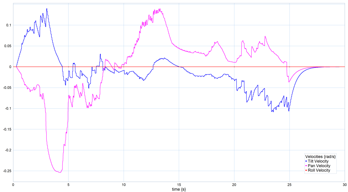
Figure 4.60: Simulated velocities while moving under a wall with patches with a limited viewing angle.
