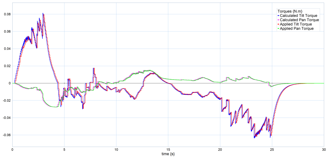
Figure 4.59: Simulated torques while moving under a wall with patches with a limited viewing angle.
