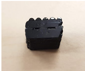
Figure 5.1: First layer of the printed three layered structure
