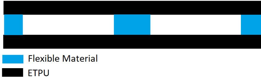
Figure 2.1: Capacitive structure where the capacitance increases when a shear force is applied. Flexibility in this sensor is higher because of the thinner flexible "walls" separating the ETPU.
