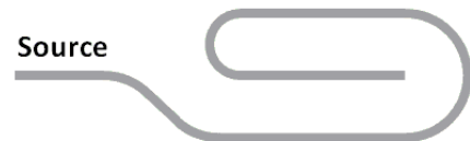
Figure 14: Sketch of the elongated spiral platinum electrodes. The left side is connected to the power source and measurement equipment.
