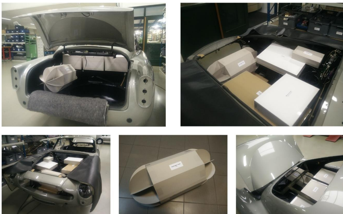
Figure 1: Cardboard models of the components placed in the car to test their position
