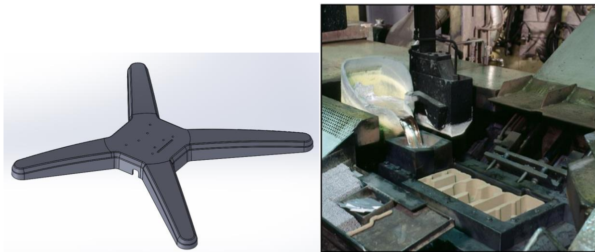
FIGURE 20: DRIVING FRAME (LEFT) & GRAVITY DIE CASTING PROCESS [5] (RIGHT)
