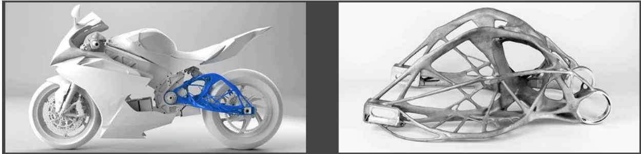
FIGURE 30: AN EXAMPLE OF A PART PRODUCED AS AN OUTCOME OF THE GENERATIVE DESIGN APPROACH [10]
