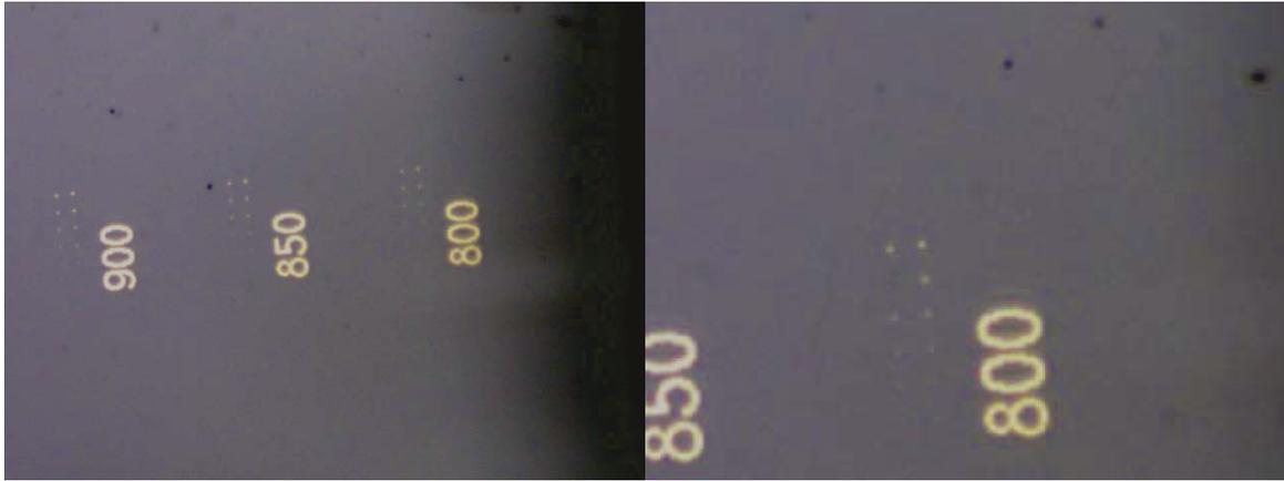
Figure 5-26 - E-Beam pattern written with different doses on BTO surface. Pictures taken with optical microscope of AFM machine. Doses are written beside each pattern.
