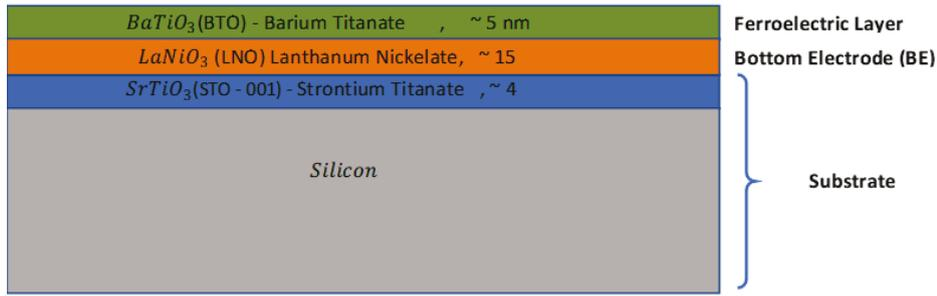
Figure 1-1 - (Above) Realizing bottom electrode and ferroelectric layer of an FTJ on single crystal  $SrTiO_3$  as main substrate and (Below) Realization of layers on STO-buffered Silicon. Above is a canonical system with reported ferroelectric property in literature.
