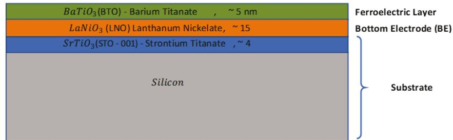
Figure 5-10 Schema of the layers deposited on top of substrate with respective thickness.
