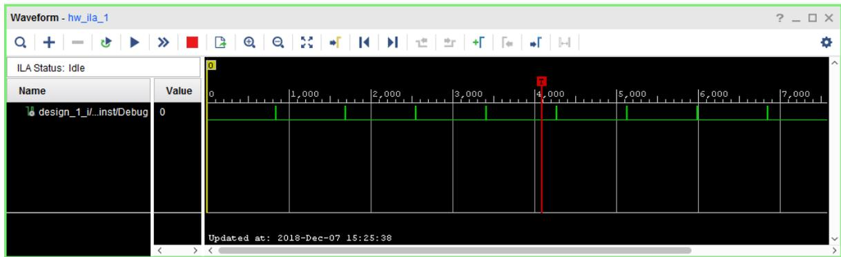
**Figure 38: Output signal indicating new data for the setup where the frequencies for the sensor and userIP are not a multiple of each other. Each pulse indicates a new output, the period between the pulses is constant meaning the output is periodic.**
