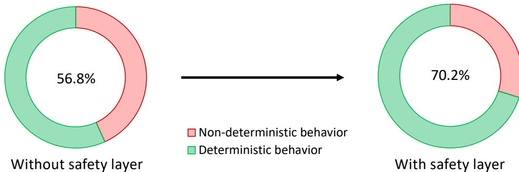
Fig. 6.8 Effect of implementing a safety layer on the probability of deterministic behavior per deployment.
