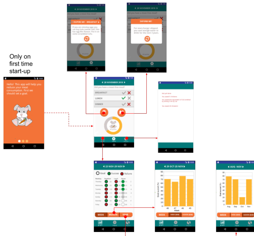
Figure 4: A diagram showing the navigation through the various pages of the app
