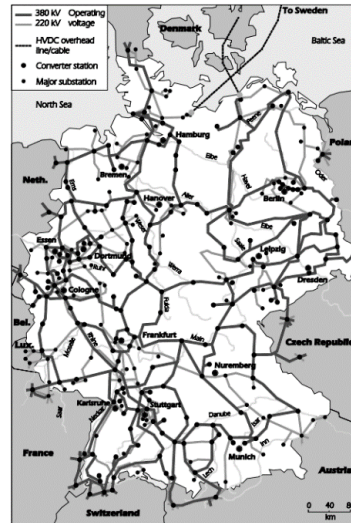
Figure 4.11 Electricity Network in Germany
