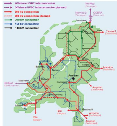
Figure 4.6 Electricity Transmission Grid in the Netherlands
