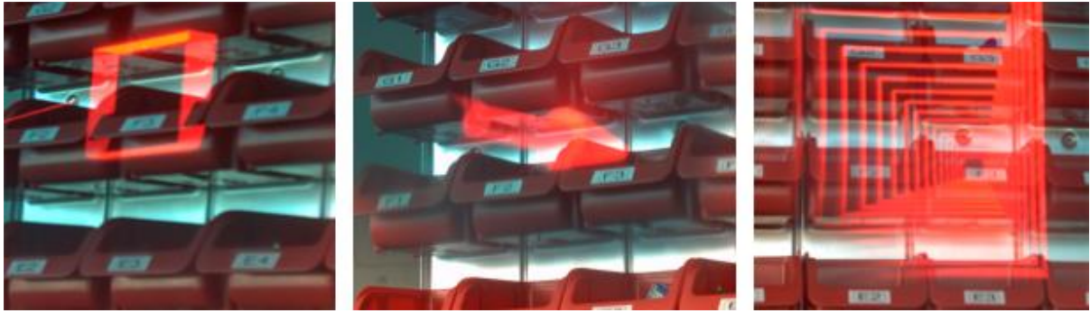
Figure 2.1 – (Left) Frame highlighting the pick bin; (Middle) Horizontal arrow pointing perpendicularly to the pick bin; (Right) Tunnel showing the pick bin. (Schwerdtfeger & Klinker, 2008).
