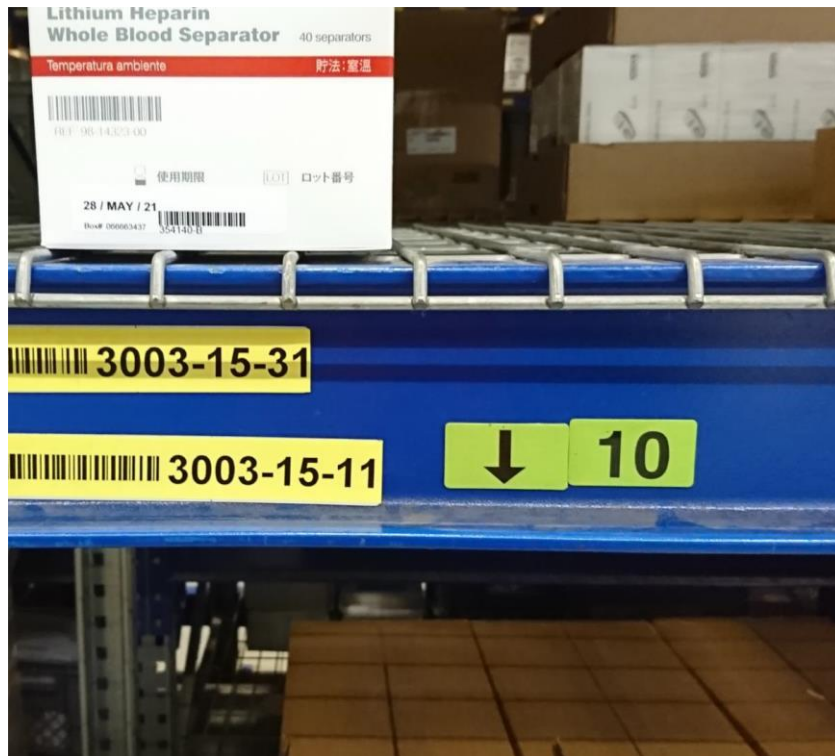
Figure 4.2 – An example of a special digit code is shown by the number ‘10’
