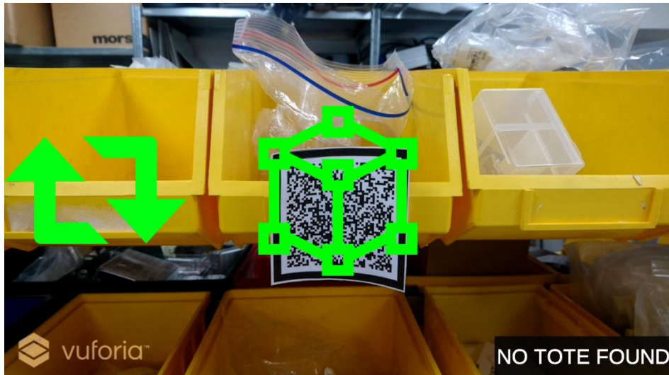
Figure 6.16 – Confirmation message when bin marker is scanned, along with the paired confirmation
