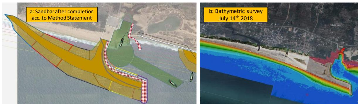
Figure 3.9: (a): Situation of the Sandbar breakwater according to the Method Statement after completion (Sand Engine excluded) (Boskalis, 2017). (b): Bathymetric survey of the Sandbar breakwater some months after completion (July 14<sup>th</sup> 2018) (Boskalis, 2018).
