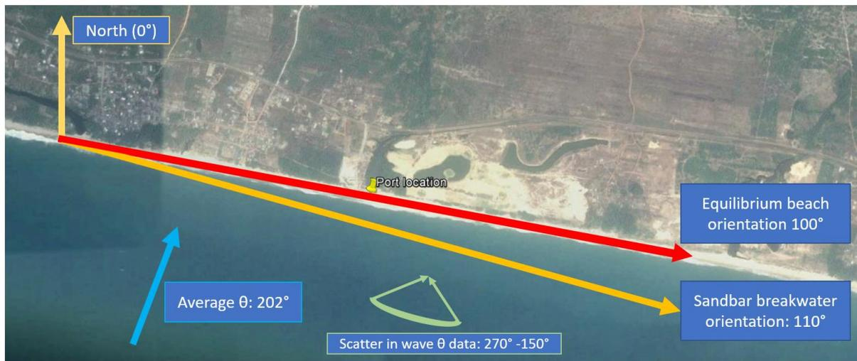
Figure 2: An overview of the initial equilibrium beach orientation ( $100^\circ$ ), the Sandbar breakwater orientation ( $110^\circ$ ), the average incoming wave direction ( $\vartheta$ ) and the scatter in incoming wave direction ( $\vartheta$ ) data obtained from the wave buoy. All orientations are expressed relative to the North ( $0^\circ$ ).
