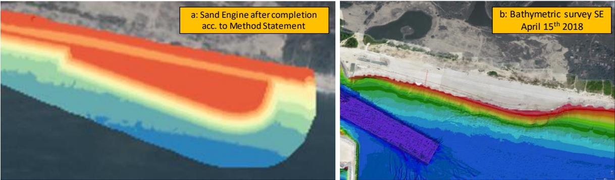
Figure 3.4: a): The design profile of the Sand Engine at the east side of the Sandbar breakwater according to the Method Statement (b): Bathymetric survey of the Sand Engine just after the completion of the Sand Engine (April 15<sup>th</sup> 2018).
