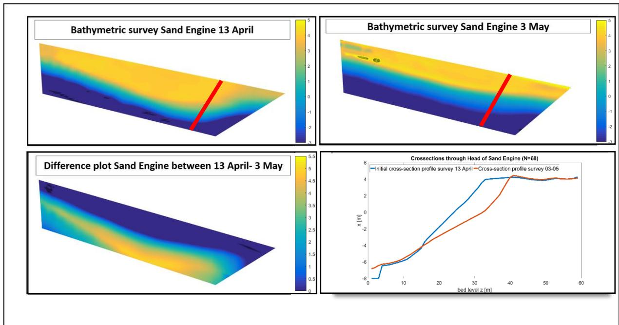
Figure 5.2: (a, top left): Top view of bathymetry survey of the Sand Engine at 13 April 2018 (b, top right): Bathymetric survey of Sand Engine at 3 May 2018 (c, bottom left): Difference plot between start and end of calibration period (d, bottom right): A cross-section through the head of the Sand Engine (located at the Sand Engine at the red line indicated in figure a, b) at start and end of calibration period (20 days, 13 April-03 May).
