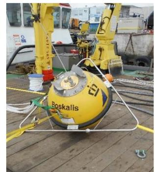
*Figure A.1: An impression of the Wave Rider used during the Lekki project*
