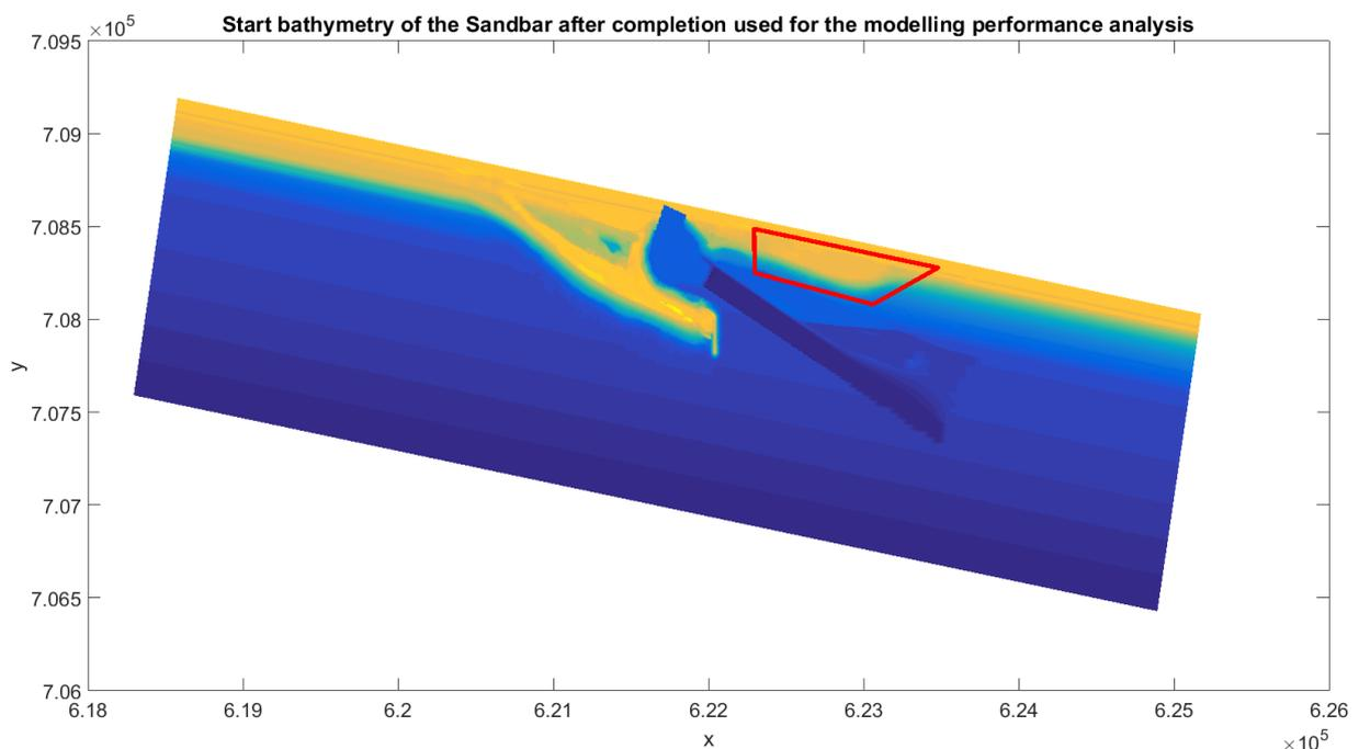
Figure 5.1: The situation of the Sandbar and Sand Engine after the completion of the Sandbar. The Sand Engine is located eastwards of the Sandbar breakwater, which is indicated by a red polygon. This area is used for the model performance study.
