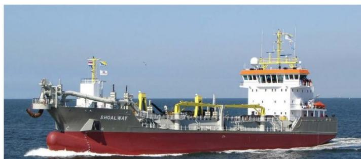
Figure B.1: The TSHD 'Shoalway', obtained from Boskalis Equipment Sheet
