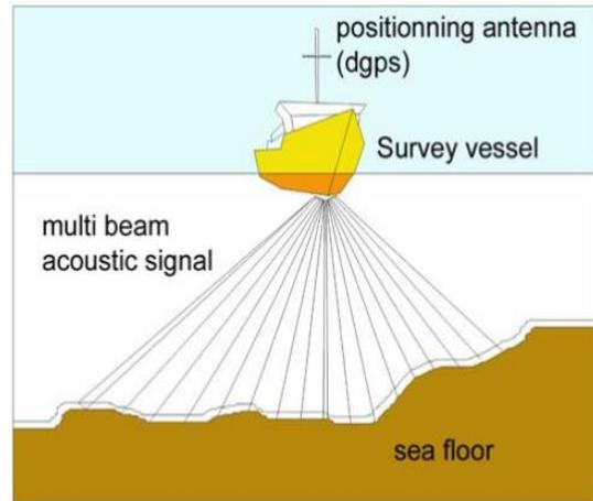
Figure A.2 A multibeam echo sounder ([www.idscope.mc/Geophy03\\_EN](http://www.idscope.mc/Geophy03_EN), retrieved: July 14<sup>th</sup>)
