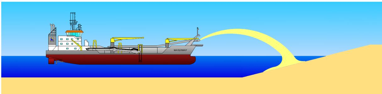
*Figure B.4: TSHD discharging via rainbow installation (Boskalis, 2017).*
