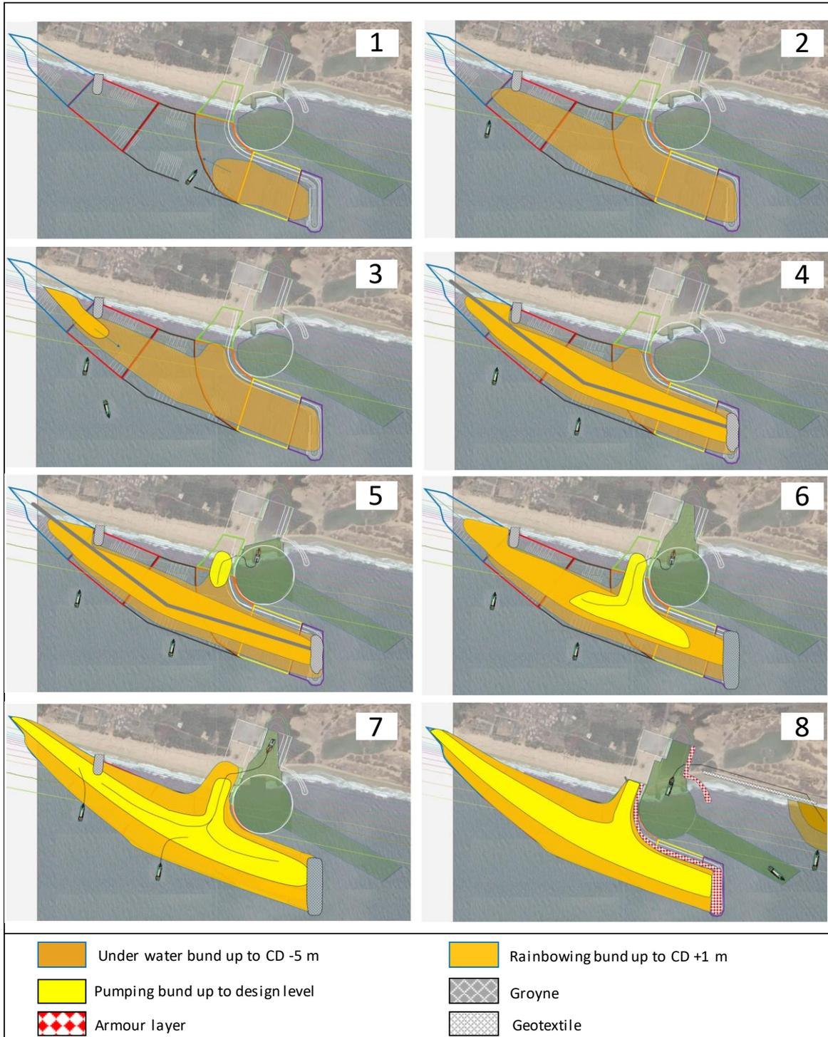
Figure 4.1: An overview of the eight stages for construction variant 1, starting with the nourishment of a submerged bund and a temporary groyne at the West side of the design profile (1,2) followed by reclamation of the Sandbar from the West (3,4). Next to that the Sandbar Road is reclaimed by a CSD (5) and subsequently the profile is further brought up to design requirements (6,7,8).
