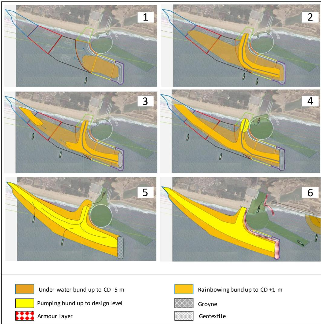
Figure 4.3: An overview of the six stages for construction variant 2, starting with the nourishment of a submerged bund and an the reclamation of the Sandbar Road followed by the 'offshore expansion' of the Sandbar from the East (3,4). Next to that the Sandbar Road is further heightened by a CSD (4) and subsequently the entire profile is further brought up to design requirements (5,6).
