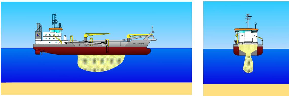
*Figure B.3: TSHD discharging at reclamation area, via bottom doors (Boskalis, 2017).*
