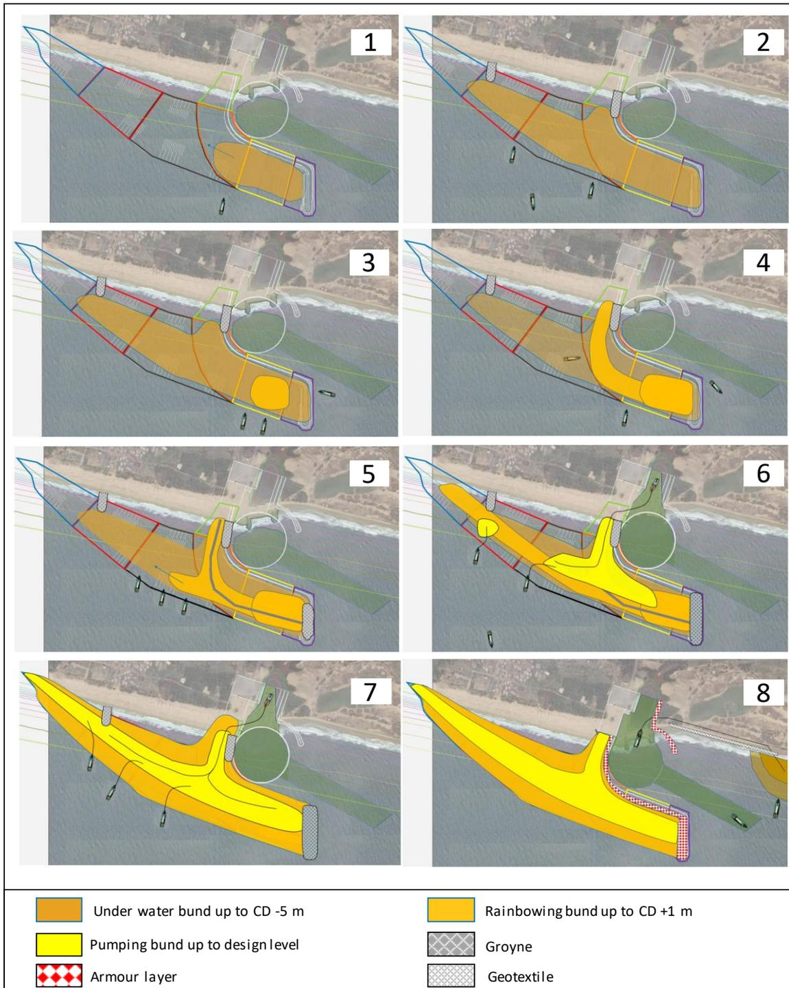
Figure 4.5: An overview of the eight stages for construction variant 3, starting with the nourishment of a submerged bund and the construction of two groyne (1,2) followed by the reclamation of an offshore island (3). Next to that the Sandbar Road is reclaimed by the TSHDs (4) and subsequently the profile is further brought up to design requirements (6,7,8).
