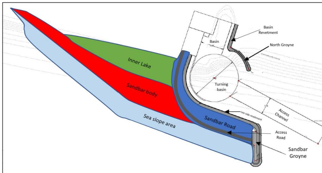
Figure 1: Overview of different components in the Lekki Sandbar breakwater design
