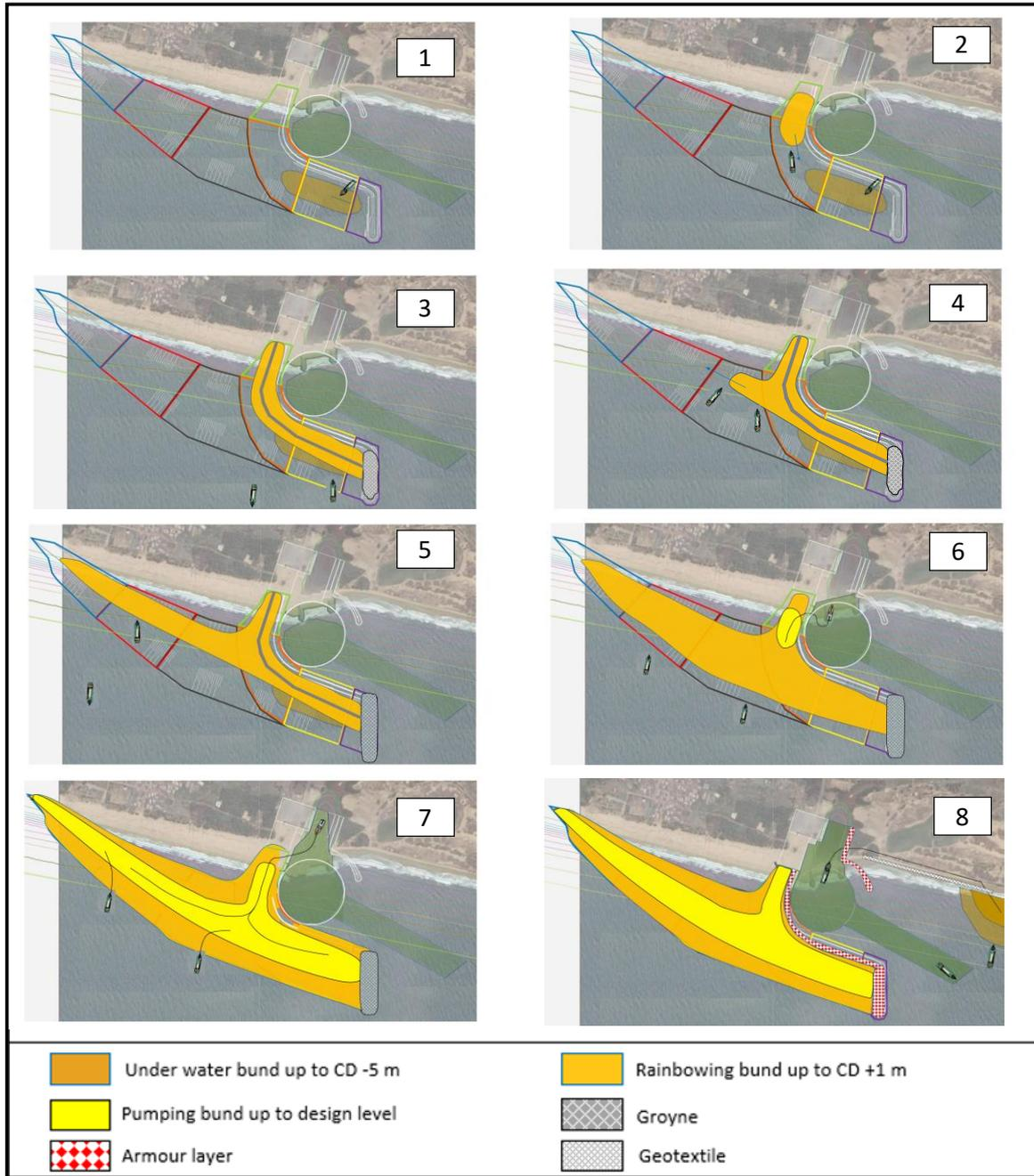
Figure A.10: An overview of the 8 stages for the generalized construction method of the Lekki project [Variant 0], starting with the nourishment of an offshore submerged bund (1) followed by the reclamation of the Sandbar Road (2). Next to that the Sandbar is reclamationed by two TSHDs (3,4,5) and subsequently the profile is further brought up to design requirements by pumping ashore (6,7,8).
