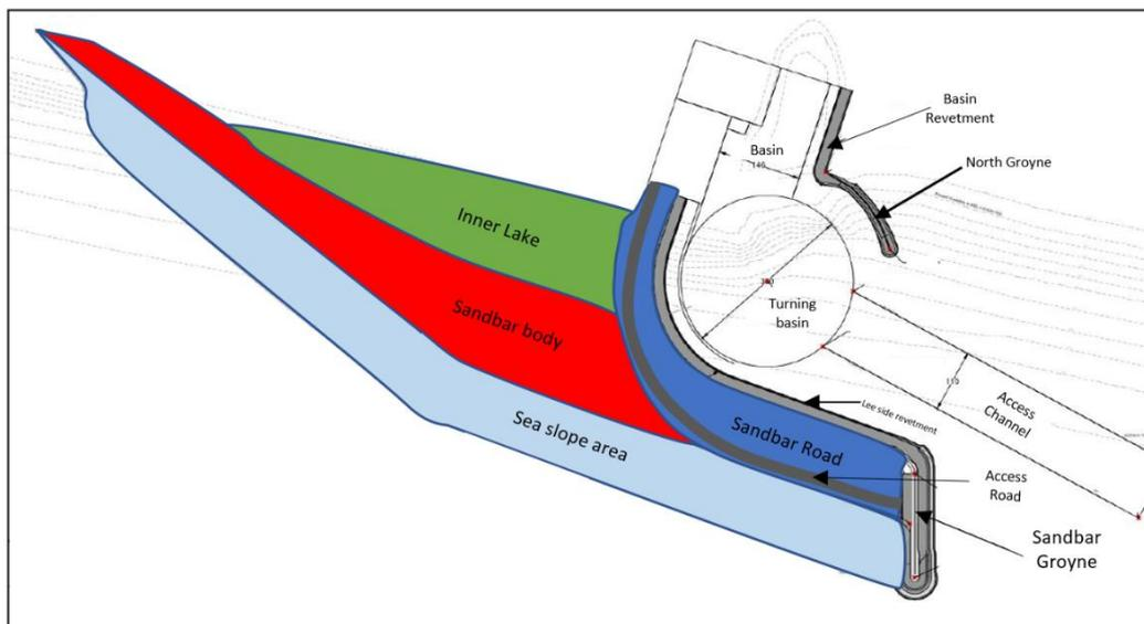
Figure 3.1: Overview of the different components in the Lekki Sandbar breakwater design
