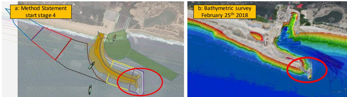
Figure 3.3: (a): Situation at the start of stage 4 according to the Method Statement showing that the construction of the Sandbar Groyne (red circle) has already started. (b): Bathymetric survey from February 25<sup>th</sup> 2018 (stage 5) showing the reclaimed Sandbar while still only a small part of the Sandbar Groyne (red circle) is constructed, implying that the construction of the Sandbar Groyne was delayed.
