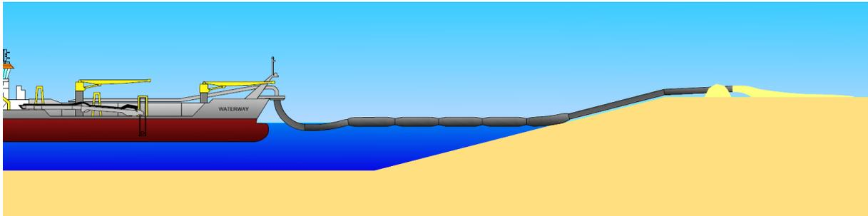
Figure B.5: TSHD discharging via floating pipeline to a reclamation area (Boskalis, 2017).
