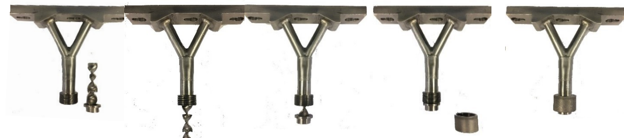
FIGURE 5.4: PROTOTYPE OF FILLING TUBE WITH STATIC MIXER
