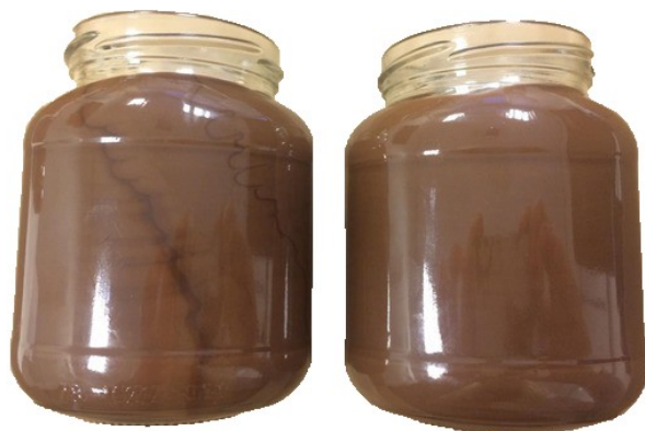
FIGURE 5.5: LEFT: WITHOUT STATIC MIXER, RIGHT: WITH STATIC MIXER
