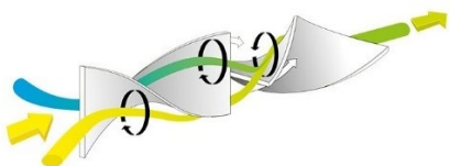
FIGURE 5.3: EXAMPLE OF A HELICAL STATIC MIXER
