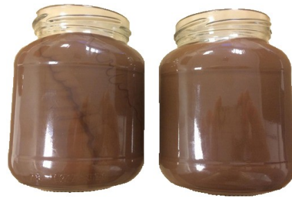
FIGURE 2: LEFT: WITHOUT STATIC MIXER, RIGHT: WITH STATIC MIXER
