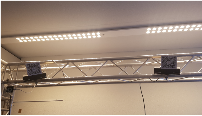
Figure 2: Kinect cameras capturing test setup from two angles.
