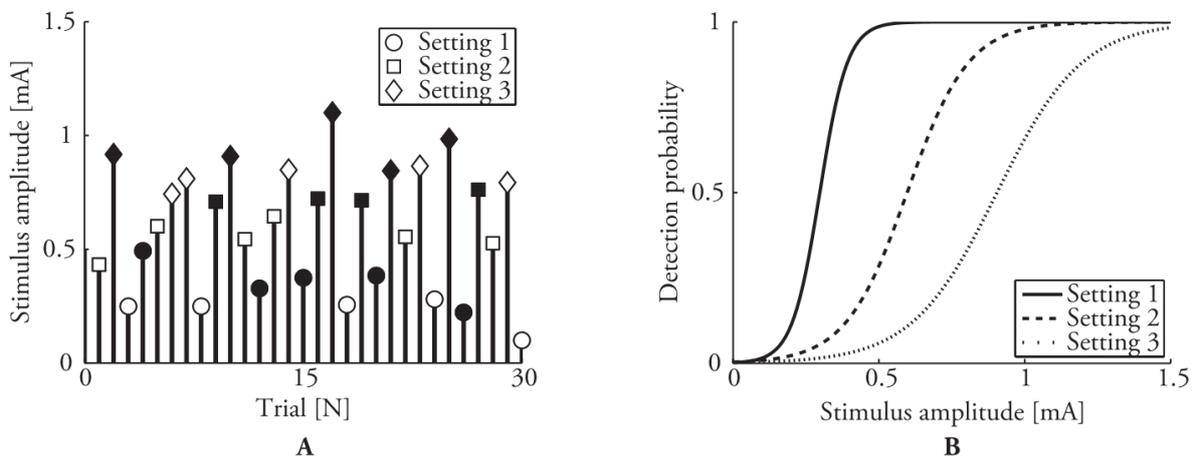
Figure 5. A). Detected (closed marker) and undetected (open marker) stimuli can be shown for each stimulus setting, when the stimulus was perceived or unperceived, respectively. B). The psychometric curve was estimated by the stimulus-response pairs from the experiment. Adapted from Doll et al. (2016).
