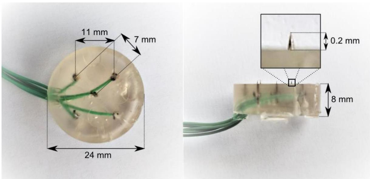
Figure 4 IES preferentially activates nociceptive nerve fibers in the superficial skin (pin-prick sensation at detection level) without initial activation of tactile nerve fibers (non-painful sensation at detection level). Therefore, IES can be used to estimate pain sensitivity measuring the NDT.
