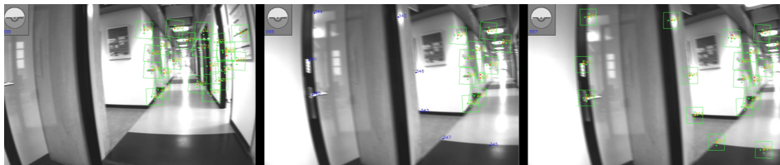
Figure 2.3: Clustering effect obtained from indoor experiment. 3 frames are shown in chronological order while the camera is moving backwards. The sequential frame number is shown in left corner.
