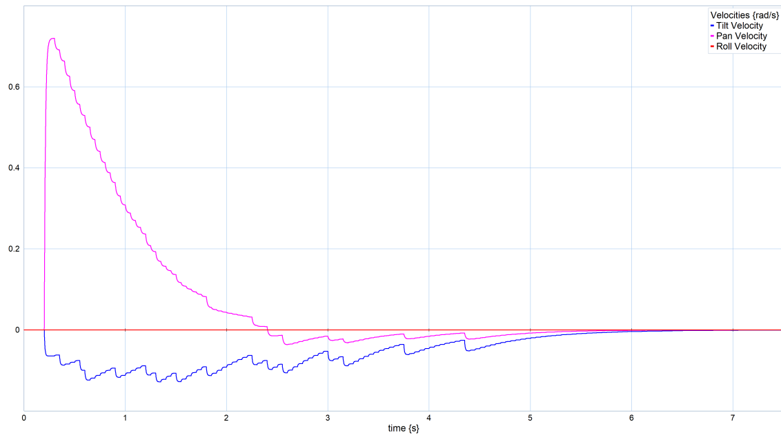
Figure 4.26: Simulated velocity response to a torus-shaped cloud of features. The camera angle includes an initial offset.
