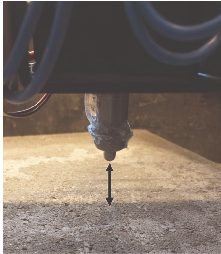
Figure 4.4: Distance between impactor and surface
