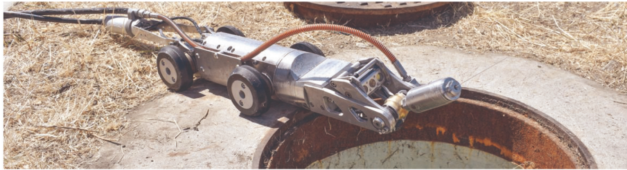
Figure 1.1: Current available sewer inspection robot of ID-tec ( https://www.id-tec.nl/ )
