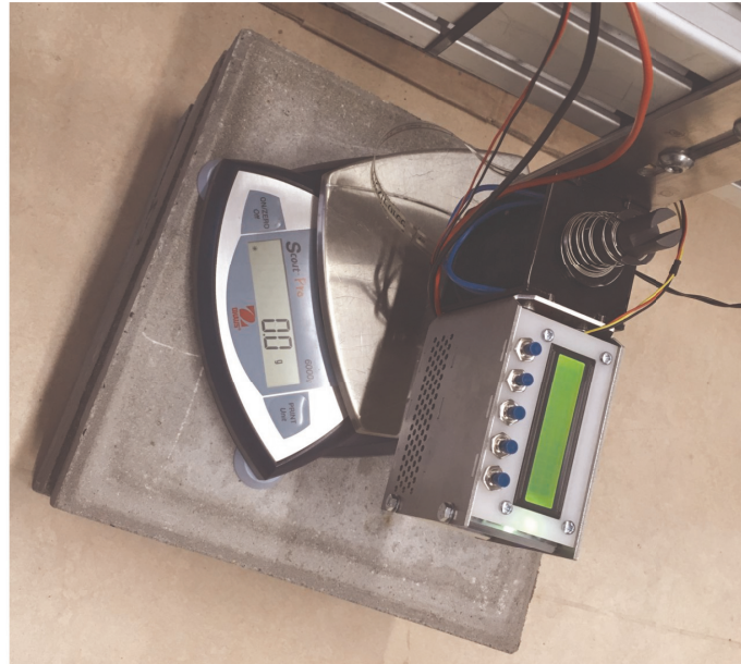
Figure 4.6: Force sensor calibration setup using scale
