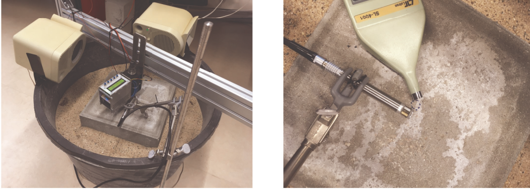
Figure 5.9: Background noise speaker placement, Figure 5.10: Background noise measurement approximately 25 cm from the sensor setup using Lutron SL-4001
