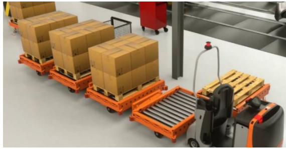
Figure 16: Milkrun System with Roller Tracks
