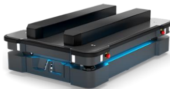
Figure 17: AGV that carries the Pallet on Top of Itself
