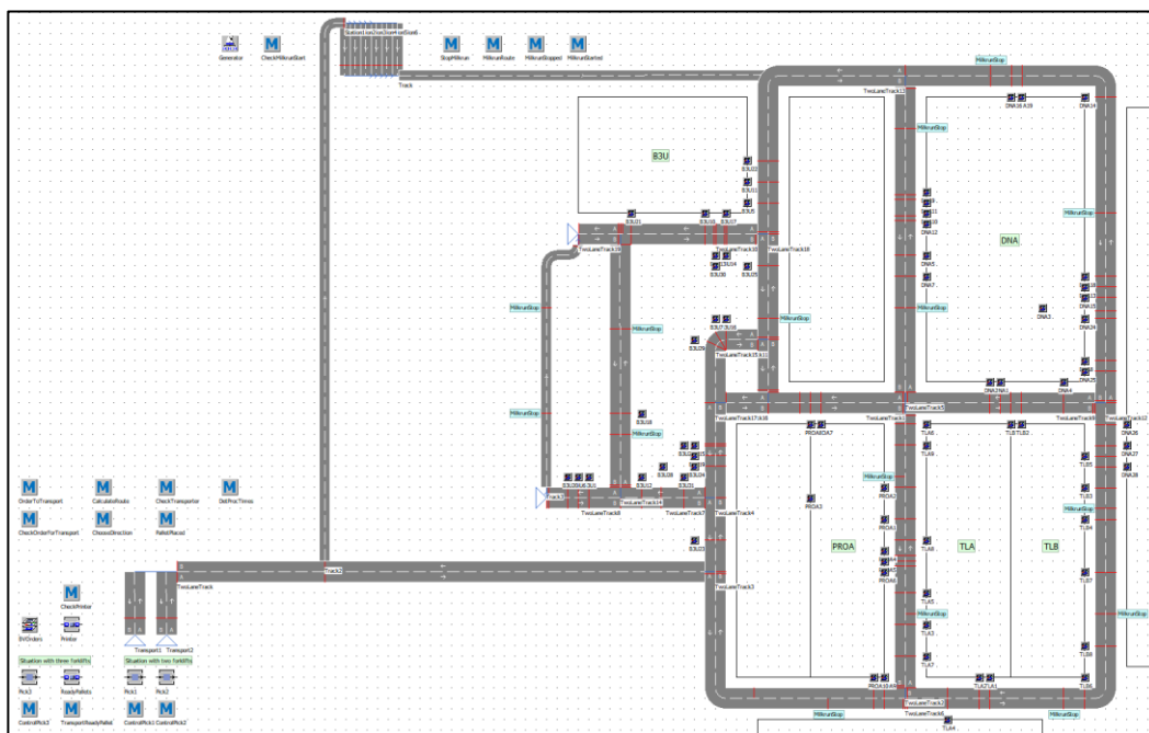
Figure 8: Layout of the Production Area in the DES Model
