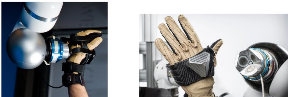
(a) The view of the connection between the hand of the human operator and the end-effector of the robotic arm when the two are in contact.
