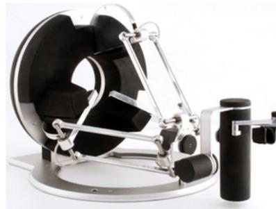
(b) The Omega.7 haptic device. From ForceDimension (2019).
