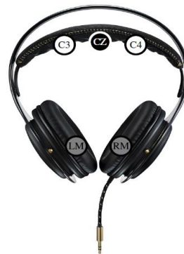
Figure 2.3: Locations of electrodes on the Philips O’Neill the Stretch 2.0 Headband Headset.
