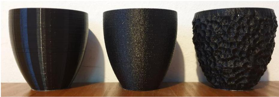
*Figure 2: The 3D printed cups (smooth vs. rough vs. rough/granular)*
