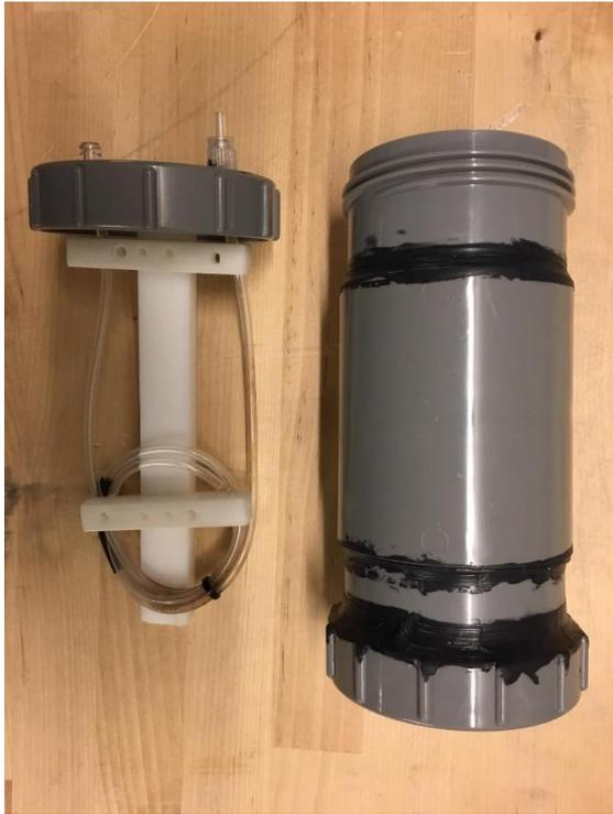
Figure 9. Flow phantom. Left: Screw cap with contrast pump tubing looping through. Right: Water filled pipe, on which the lid can be screwed.
