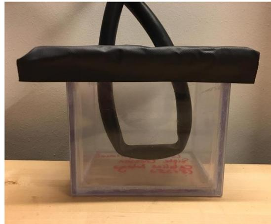
Figure 3. Water tank with the 13 mm tube looping through the lid of the tank.
