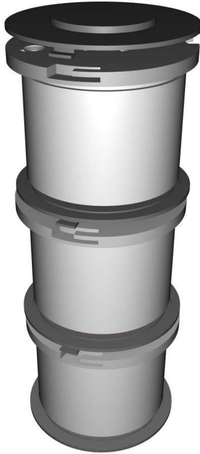
Figure 19: A 3D view of all elements together forming the phantom case design with the three segments.
