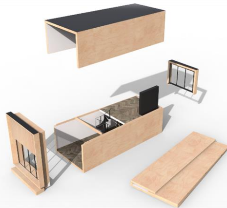
Figure 4: Exploded view of attachable and foldable parts (D'Andrea & Evers, 2018).
