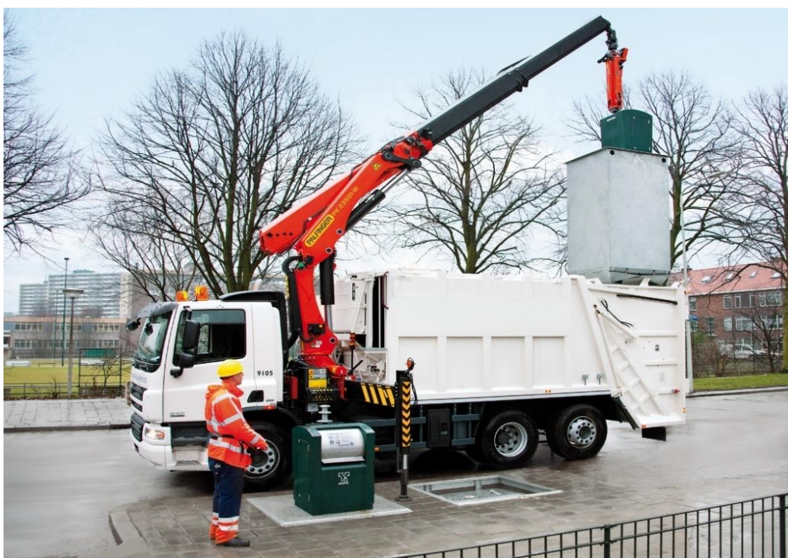
Figure 3: Emptying an underground waste container (photo credit: Palfinger.ag)
