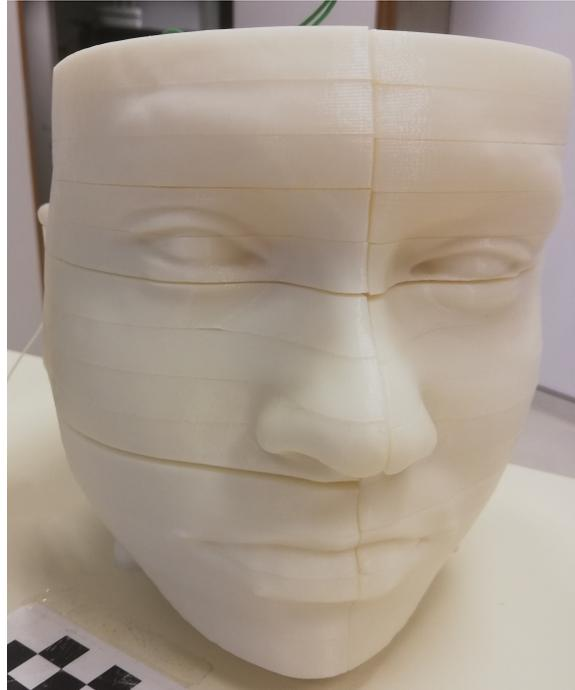
Figure 14: The 3D printed phantom
