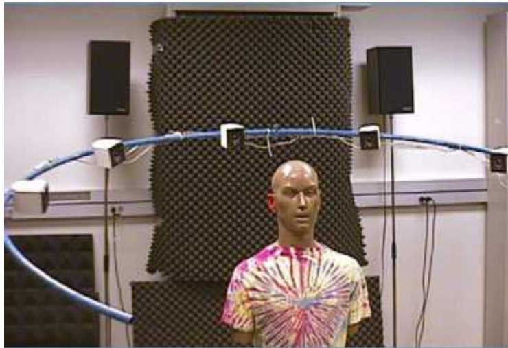
Figure 4. HRIR measurements using KEMAR 1
