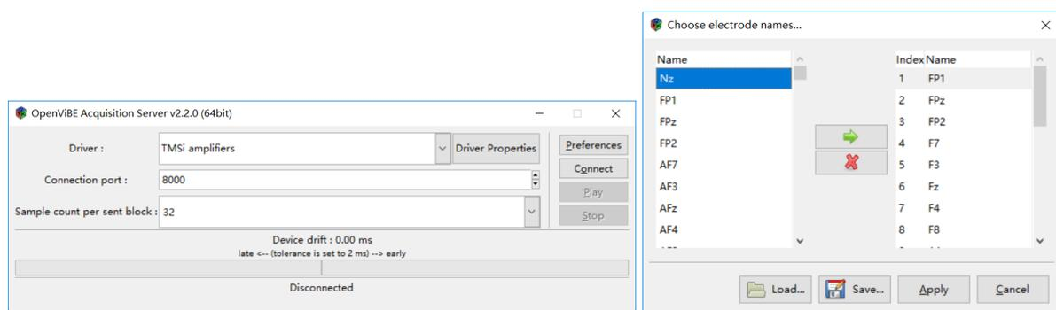
(a) Driver and connection port setting of the OpenVibe acquisition window (b) Maps between electrode name and index
