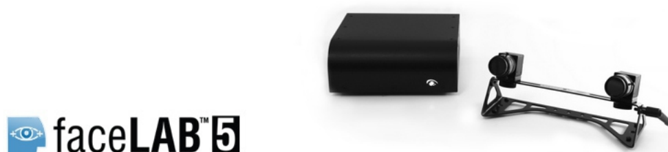
Figure 2.6: FaceLAB 5 eye tracking system by Seeing Machines, retrieved from (ekstremakina, n.d.)
