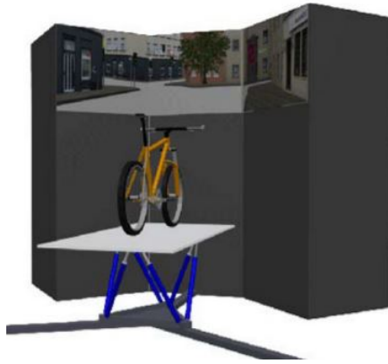
Figure 2.10: FIVIS setup, retrieved from (Schulzyk, Hartmann, Bongartz, Bildhauer & Herpers, 2009)
