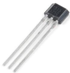
Figure 5.15: A linear Hall effect sensor.<sup>21</sup>
