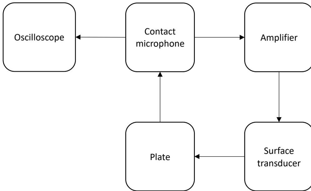
Figure 6.6: Block diagram of the setup of experiment 1, the arrows signify the travel of sound.
