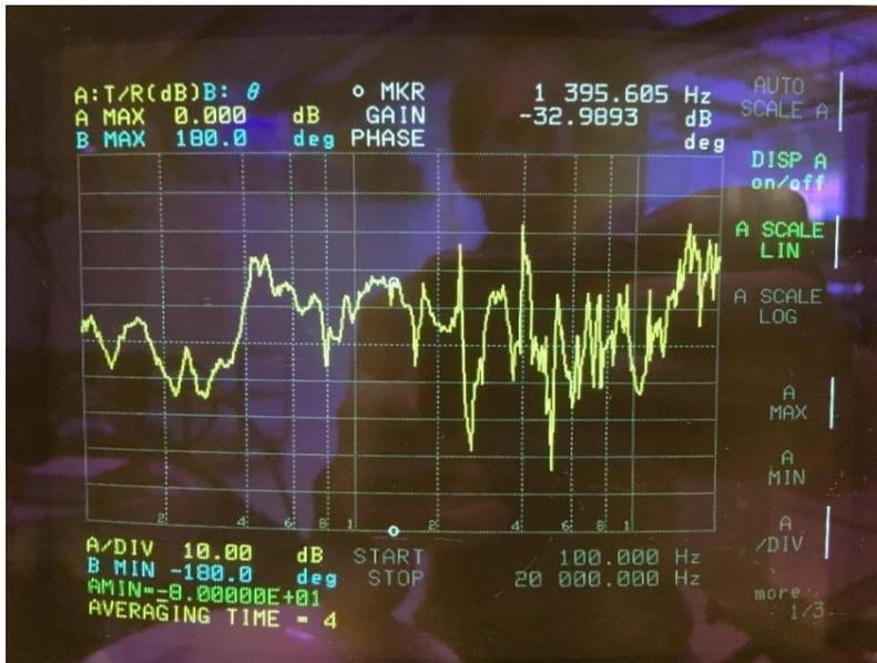
Figure A2.0.7: Large surface transducer on plate at 20dB attenuation, small piezo.
