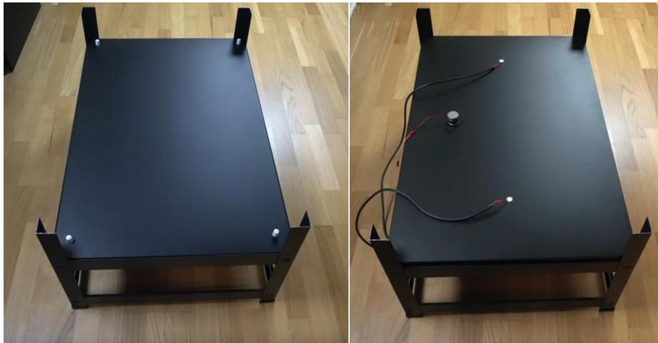
Figure 5.5: Bottom plate with spacers on the left, top plate with surface transducer and contact microphones on the right.<sup>15</sup>
