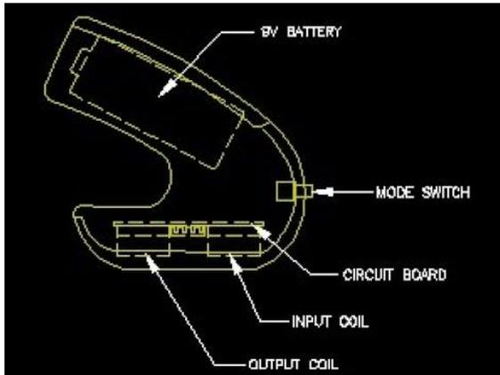
Figure 2.3: a high-level overview of an EBow.<sup>4</sup>
