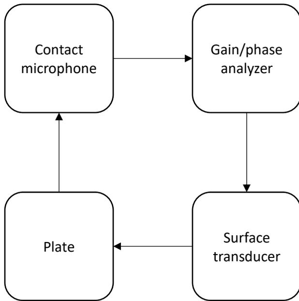
Figure 6.8: Block diagram of the setup of experiment 2, the arrows signify the travel of sound.
