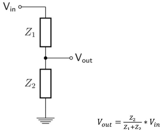
Figure 5.23: A schematic of a voltage divider. In the case of an amplifier input, its input impedance is  $Z_2$ . This means that the lower its value, the lower  $V_{out}$  will be.
