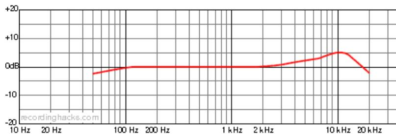
Figure 5.12: frequency response curve of the Studio Projects B1.<sup>19</sup>
