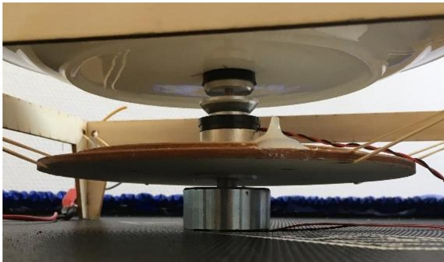
Figure A3.0.2: Stack of surface transducers, with the bottom one resting on the trampoline.
