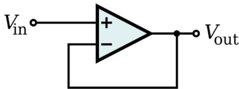
Figure 5.24: Operational Amplifier in buffer configuration.
