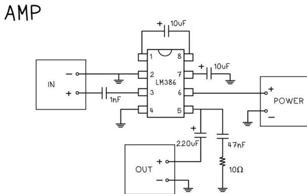
Figure 5.22: circuit of Evan Kale's tin can amplifier build.<sup>25</sup>
