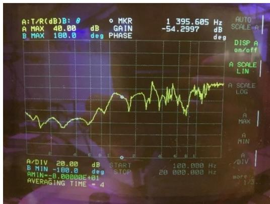
Figure A2.0.8: Medium Surface transducer on plate at 0dB attenuation, small piezo.
