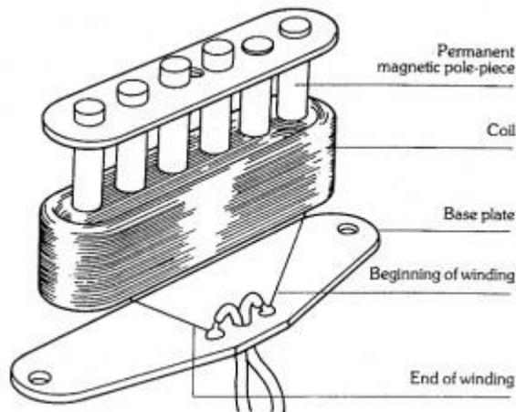
Figure 5.13: Inside of a single coil guitar pickup.<sup>20</sup>
