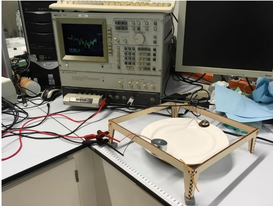
Figure A2.0.1: One of the used test setups, this iteration with a large surface transducer and a large piezo disc.
