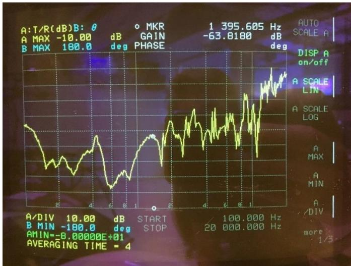
Figure A2.0.5: Medium surface transducer on plate at 20dB attenuation, large piezo.
