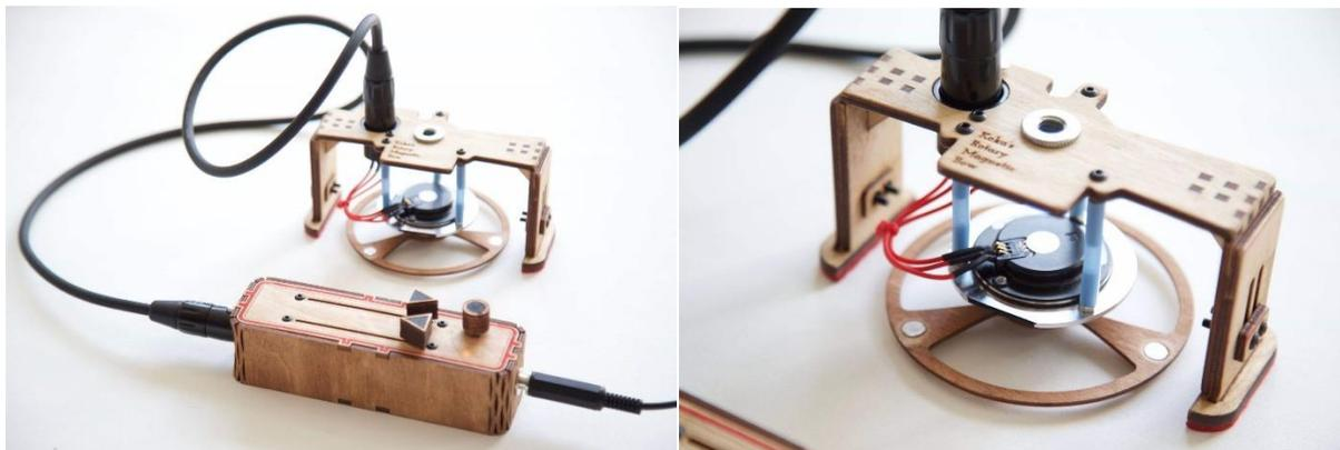
Figure 2.6: Left: Koka's Rotary Magnetic Bow full setup, right: close-up shot of the rotary bow.<sup>7</sup>
