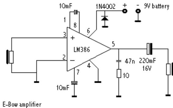
input coil: use telephone pick-up
