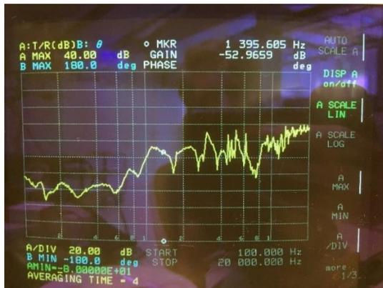
Figure A2.0.9: Medium Surface transducer on plate at 20dB attenuation, small piezo.
