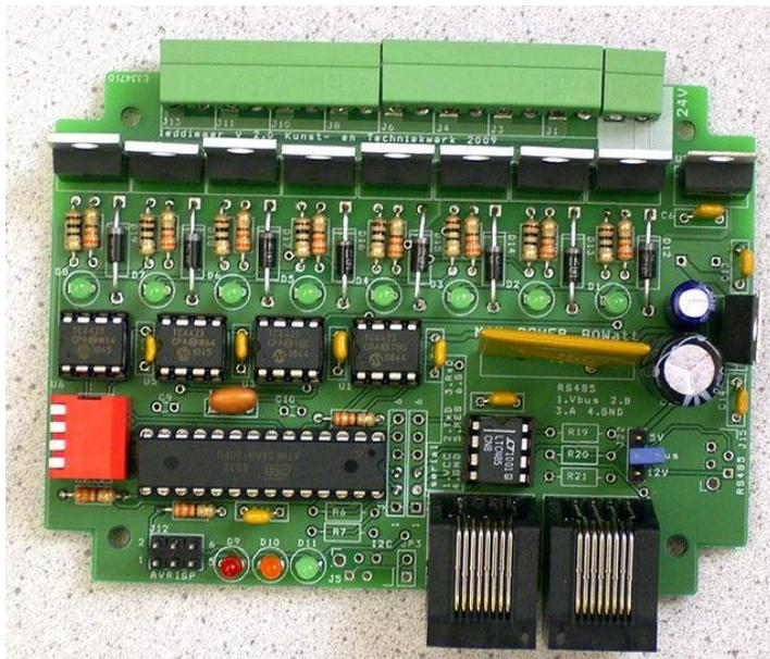
Figure 2.1: Edwin Dertien's 24V LED dimmer board.<sup>2</sup>
