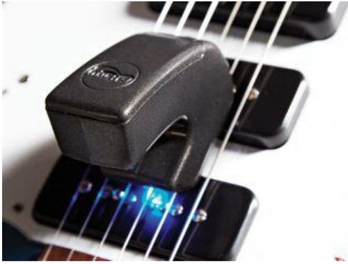
Figure 2.2: An EBow placed on an electric guitar.<sup>3</sup>
