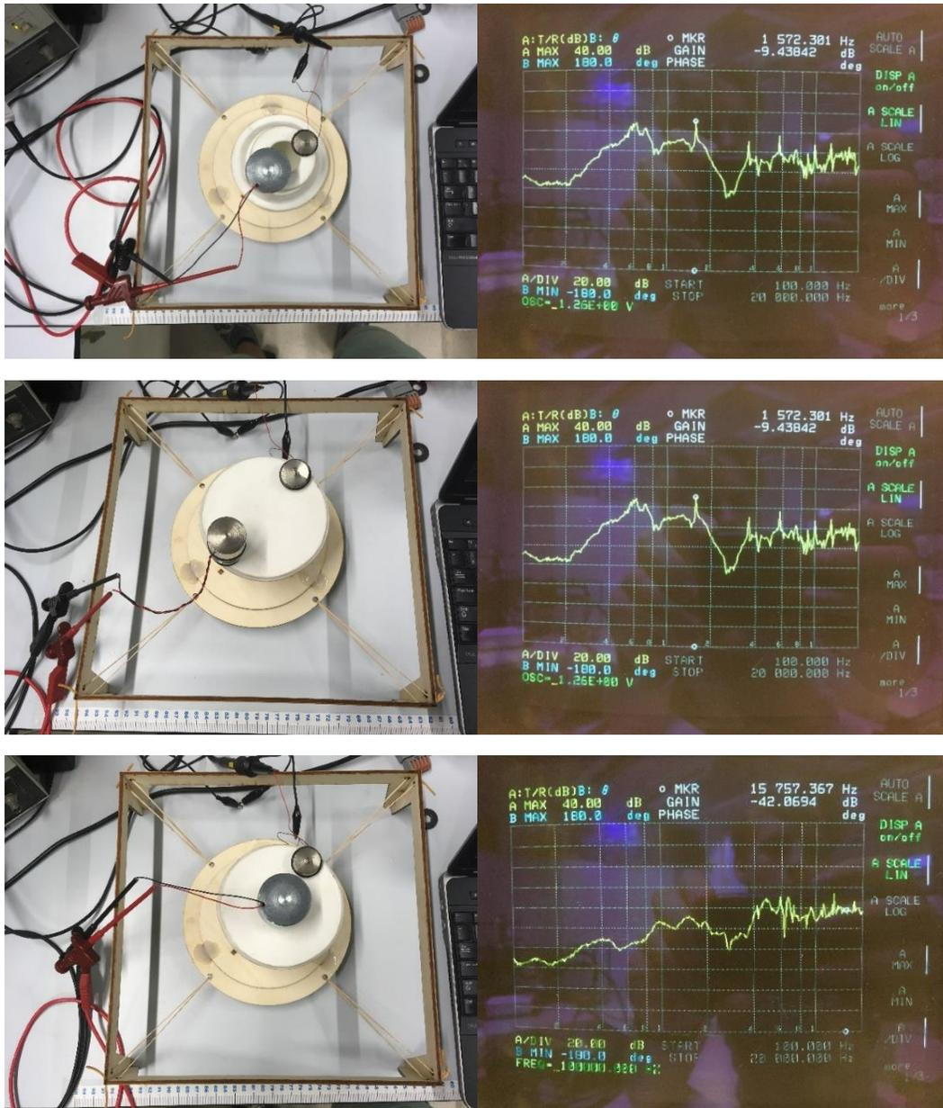
Figure A2.0.11: Impact of placement of surface transducer on produced bode plot for the ceramic artifact.
