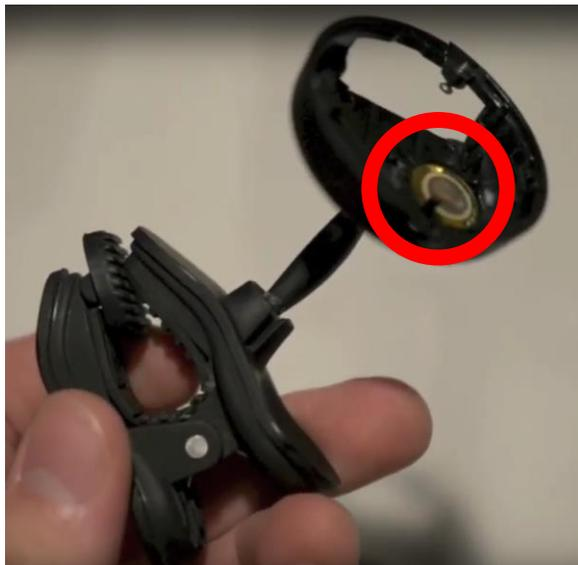
Figure 5.18: The inside of a Snark clip-on tuner, with the location of the piezo disc clearly visible.<sup>24</sup>
