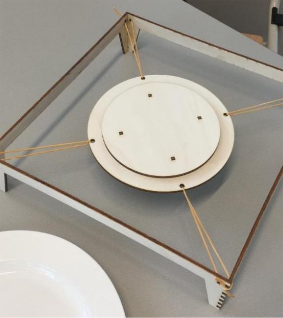
Figure 6.2: shock mount test setup for ceramic plate.
