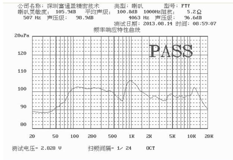
Figure 5.9: Adafruit Medium Surface Transducer frequency response graph [37]. The large 'PASS' means that this transducer passed some sort of quality control, it has nothing to do with filtering.
