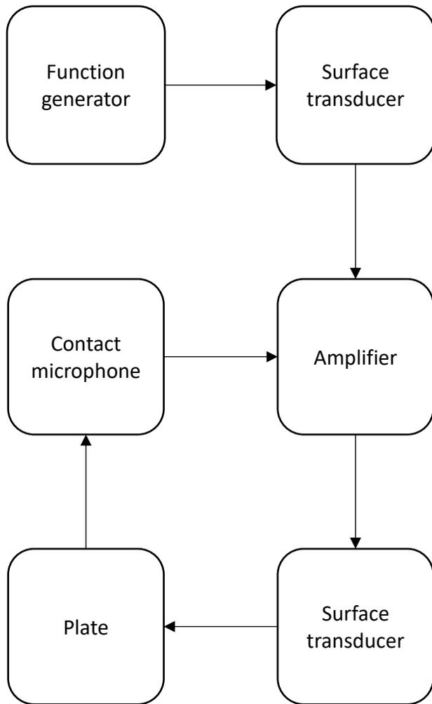
Figure 6.10: Block diagram of the setup of experiment 3, the arrows signify the travel of sound.
