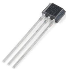
Figure 5.15: A linear Hall effect sensor.<sup>21</sup>
