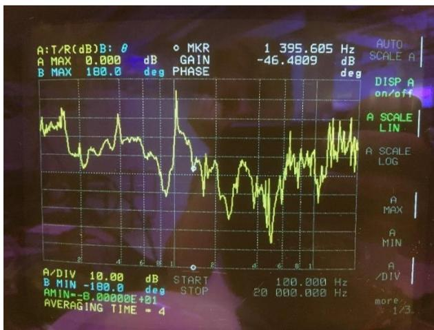
Figure A2.0.3: Large Surface transducer on plate at 0dB attenuation, large piezo.
