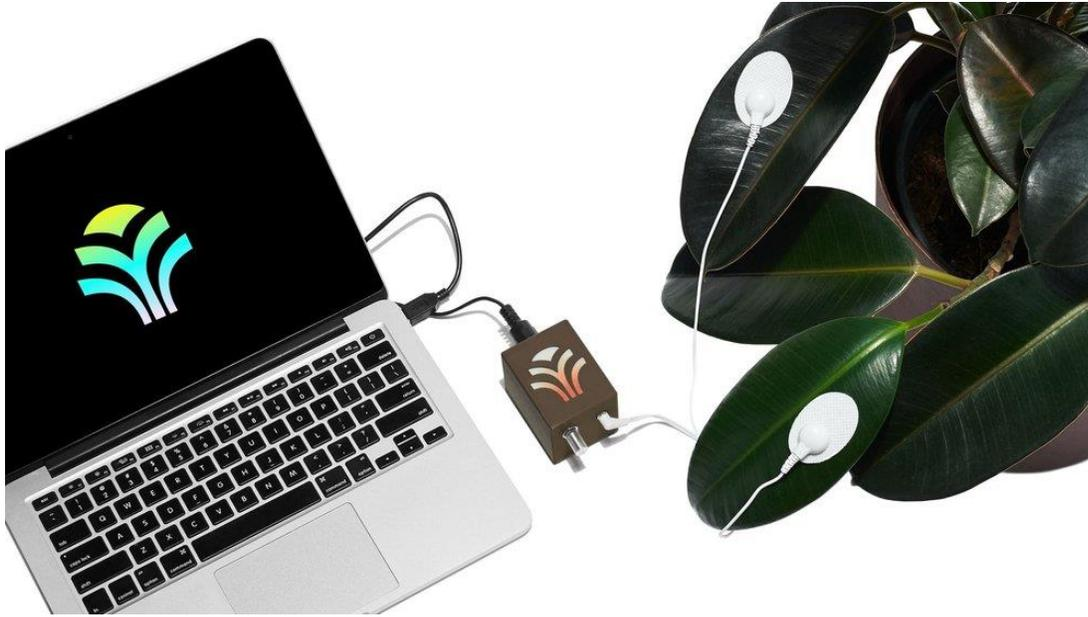
*Figure 2.10: MIDI Sprout interfaced with a MacBook Pro via MIDI over USB and electrodes placed on a plant as input.<sup>11</sup>*
