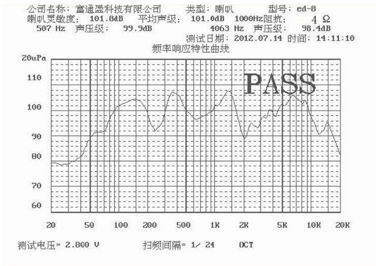
Figure 5.10: Adafruit Large Surface Transducer frequency response graph [38].
