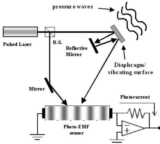
figure 5.14: Setup of a laser microphone [39].
