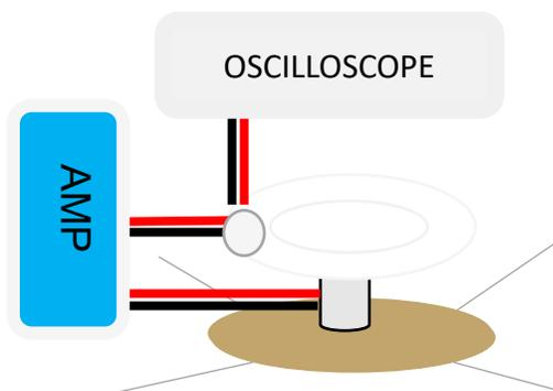
Figure 6.5: Graphical overview of the block diagram of the setup in experiment 1.
