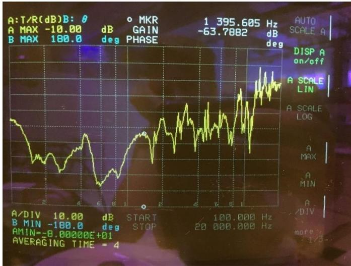
Figure A2.0.4: Medium surface transducer on plate at 0dB attenuation, large piezo.
