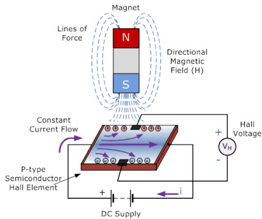
Figure 5.16: Diagram that shows how a Hall effect sensor works.<sup>22</sup>
