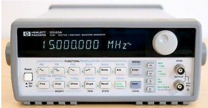
Figure 5.25: HP 33120A function generator.
