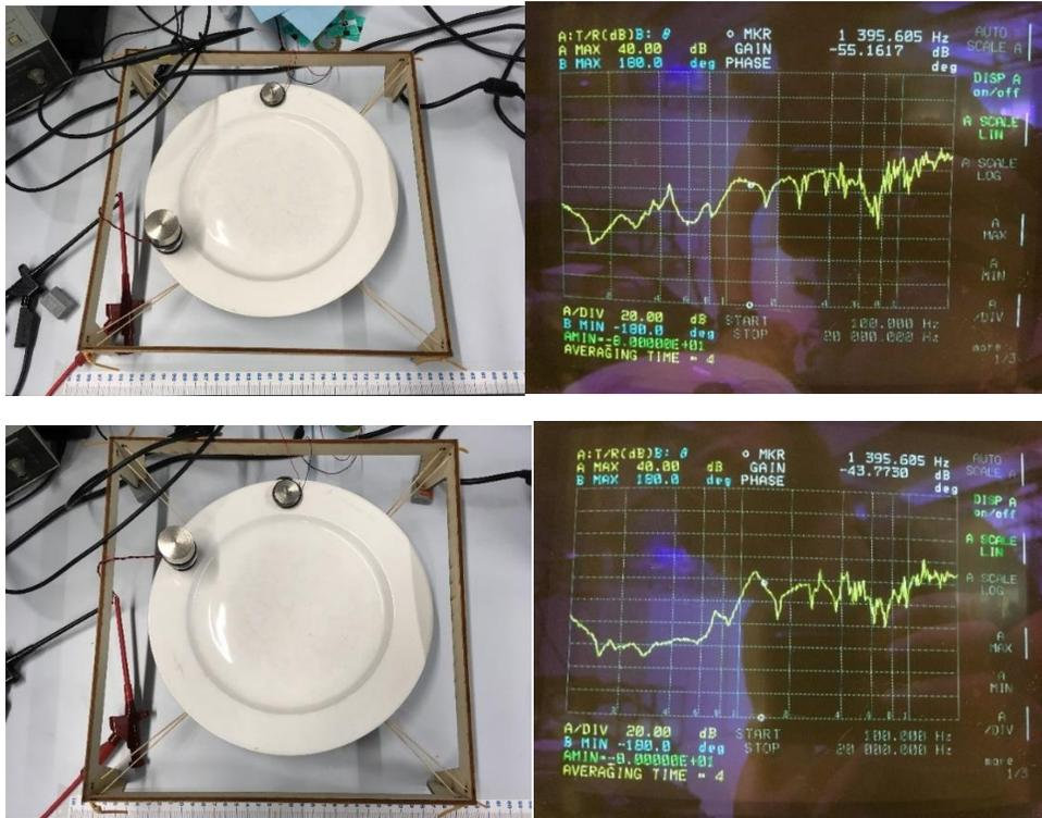
Figure A2.0.10: Influence of placement of the surface transducer on the produced bode plot.
