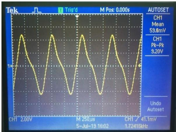
Figure A1.0.4: Oscilloscope view of the produced audio feedback using the large surface transducer.
