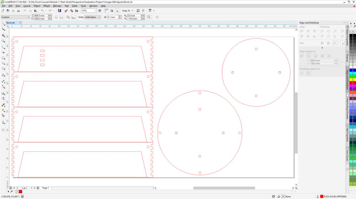
Figure 6.3: CorelDRAW X7 design file of the shock mount.
