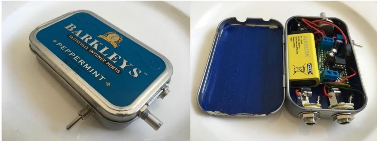
Figure 5.21: A build of Evan Kale's tin can amplifier.
