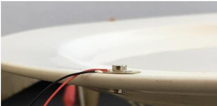
*Figure A1.0.1: Mounting the piezo disc mounted on the rim of the dinner plate.*
