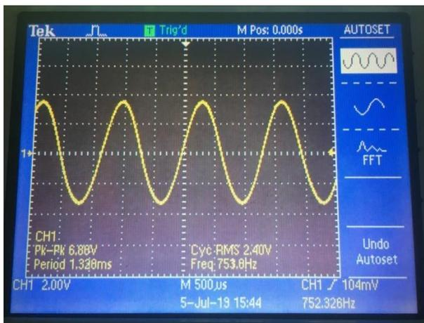
Figure A1.0.3: Oscilloscope view of the produced audio feedback using the medium surface transducer.
