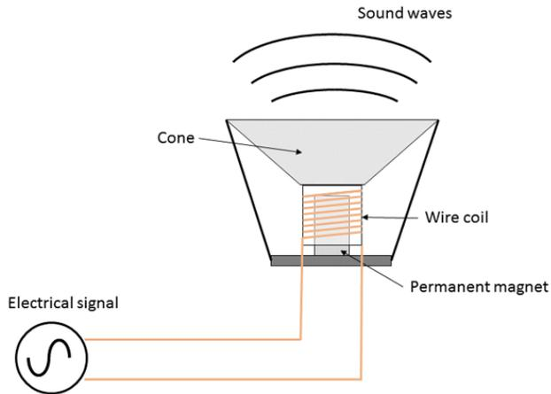
Figure 5.4: Simplified anatomy of a standard loudspeaker.<sup>14</sup>
