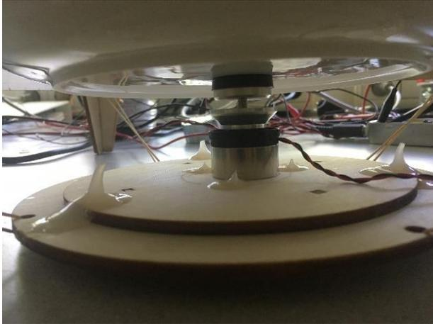
Figure A1.0.2: Placing the surface transducer under the plate.
