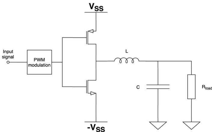
Figure 2.1: Schematic of an ideal class D amplifier with a second order filter and resistive load
