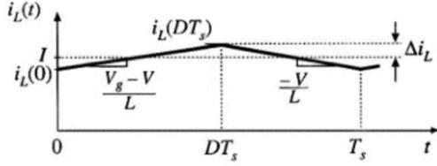
Figure 2.3: *Steady-state inductor current waveform [1]*
