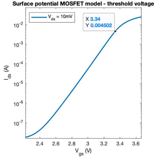
Figure 4.7: Logarithmic plot of  $I_{ds}$  versus  $V_{gs}$  for  $V_{ds} = 10\text{mV}$  of a standard surface-potential based MOSFET model to determine  $V_{th}$
