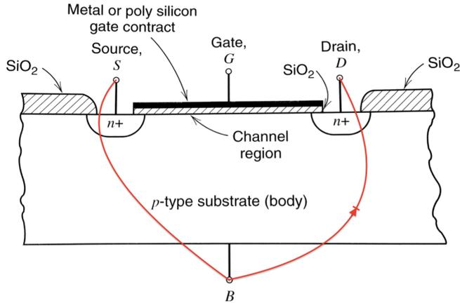
Figure 4.1: *NMOS simplified internals [2] with the body diode connections in red annotation*
