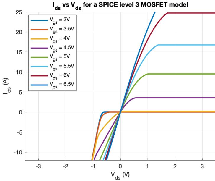
Figure 4.5:  $I_{ds}$  versus  $V_{ds}$  for different  $V_{gs}$  of a level 3 MOSFET model
