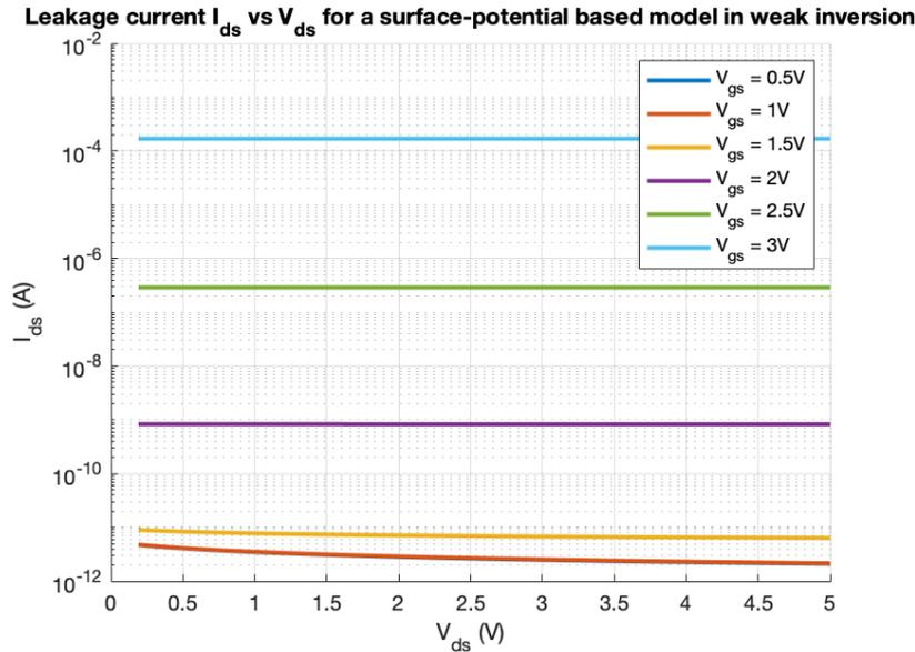
Figure 4.8:  $I_{ds}$  versus  $V_{ds}$  for different  $V_{gs}$  of a surface-potential based MOSFET model in weak inversion (i.e. for  $V_{gs}$  below  $V_{th}$ ). Note:  $V_{gs} = 0.5\text{V}$  and  $V_{gs} = 1\text{V}$  are very close to each other
