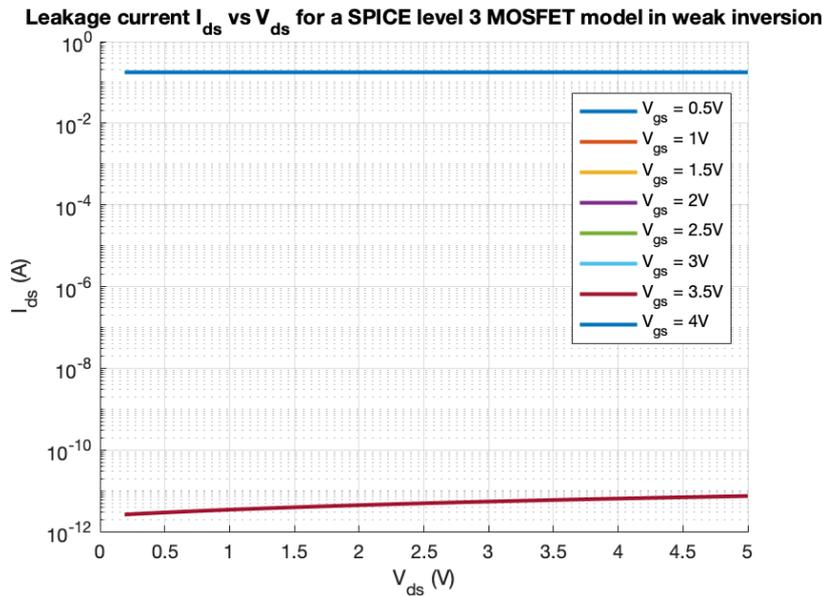
Figure 4.4:  $I_{ds}$  versus  $V_{ds}$  for different  $V_{gs}$  of a level 3 MOSFET model in weak inversion (i.e. for  $V_{gs}$  below  $V_{th}$ ). Note:  $V_{gs} = 0.5V$  up until  $V_{gs} = 3.5V$  are all the same line. Only  $V_{gs} = 4V$  is separated, since this is above  $V_{th} = 3.88V$
