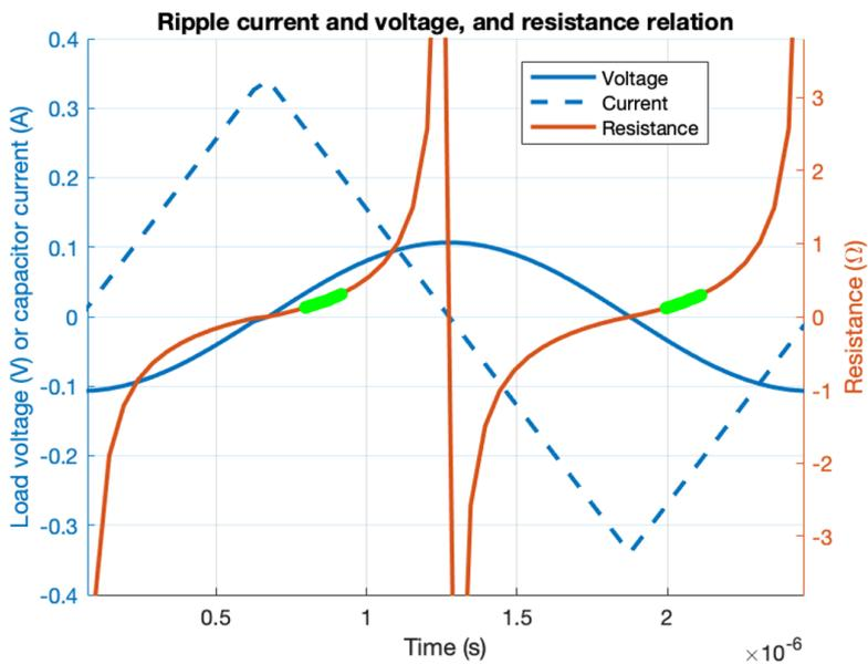
Figure 5.5: The voltage over the load (blue), the current absorbed by the capacitor (blue dotted) and the division of both expressed in Ohms (orange). In green the resistor values are marked that the MOSFET can create.
