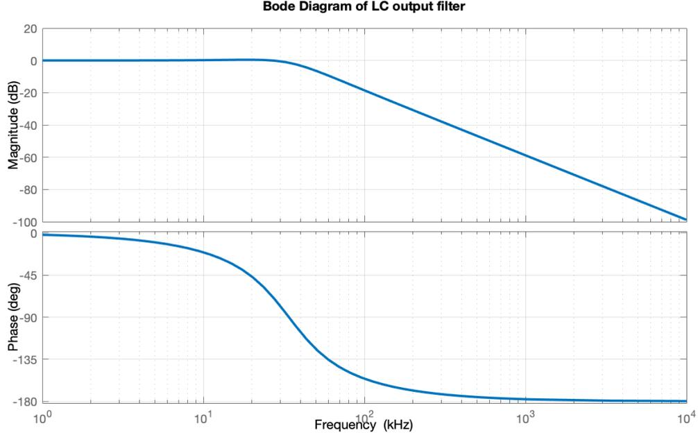
Figure 2.2: *Phase and magnitude plots versus frequency for the LC output filter with  $L = 22\mu H$  and  $C = 1\mu F$*
