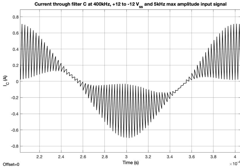
Figure 5.2: *Current through the capacitor of the class D amplifier of figure 2.1 with AC input signal*
