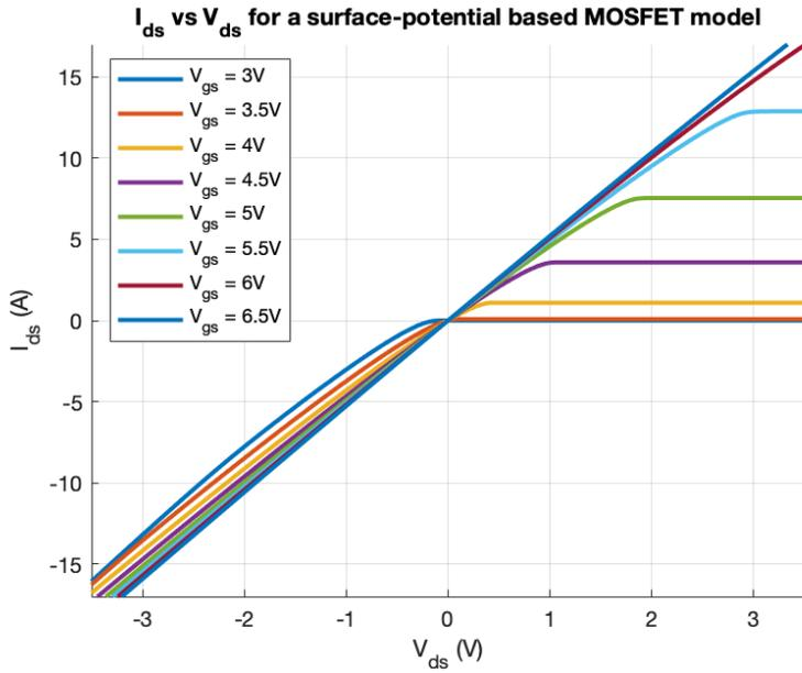
Figure 4.9:  $I_{ds}$  versus  $V_{ds}$  for different  $V_{gs}$  of a standard surface-potential based MOSFET model
