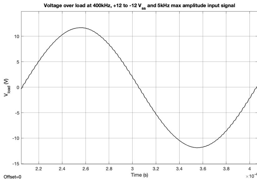
Figure 5.1: *Voltage over the load of the class D amplifier of figure 2.1 with AC input signal*
