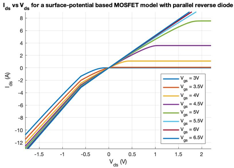
Figure 4.12:  $I_{ds}$  versus  $V_{ds}$  for different  $V_{gs}$  of a surface-potential based MOSFET model with a diode in parallel as shown in figure 4.11
