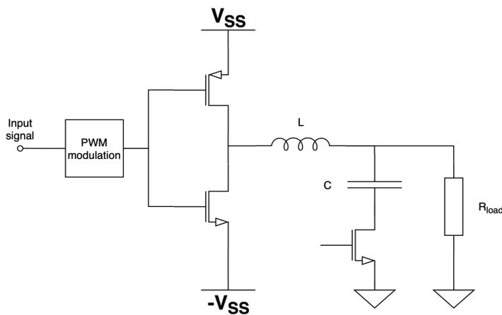
Figure 3.1: Class D amplifier from figure 2.1 with a FET added in series with the capacitor
