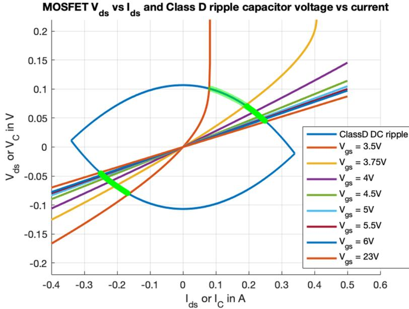
Figure 5.4: *The voltage-current combinations of a surface-potential based MOSFET model and the voltage-current combinations of the ripple in the capacitor of a class D amplifier*
