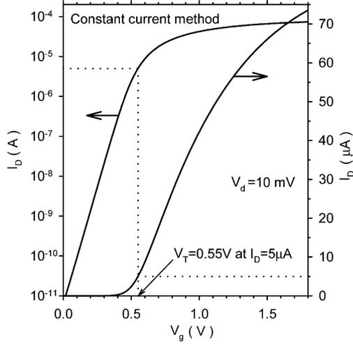
Figure 4.2: Constant current method as described by Ortiz-Conde et al. [3]. The dotted line shows the location on both the logarithmic and linear curve for the threshold voltage.
