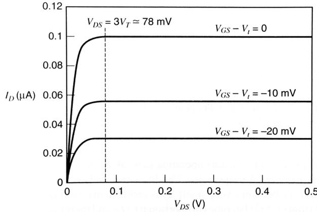
Figure 4.3:  $I_{ds}$  versus  $V_{ds}$  for different  $V_{gs}$  below threshold [2], according to equation 4.1
