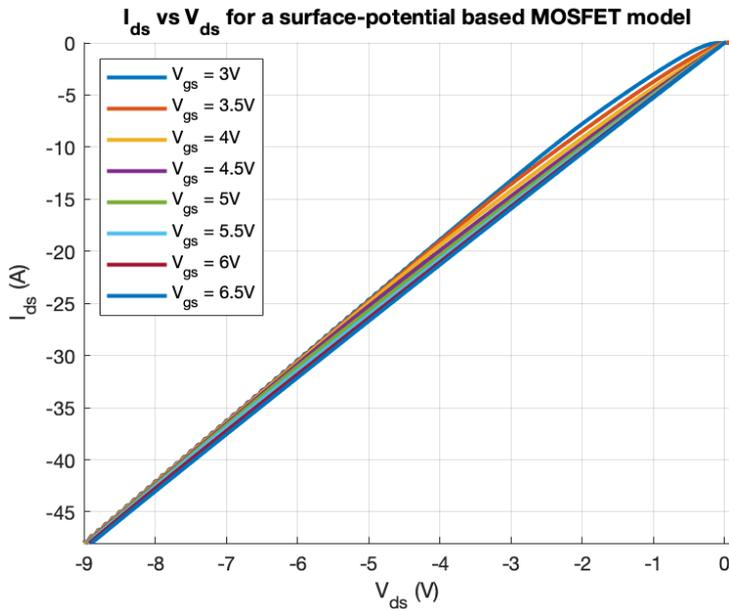
Figure 4.10:  $I_{ds}$  versus negative  $V_{ds}$  for different  $V_{gs}$  of a standard surface-potential based MOSFET model
