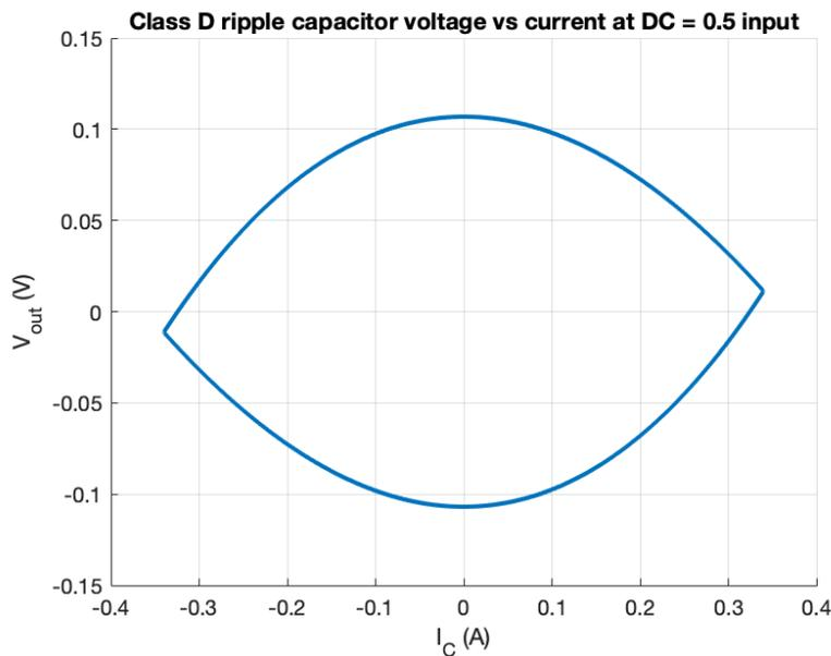
Figure 5.3: *Current versus voltage through the capacitor of the class D amplifier of figure 2.1 with DC input signal*
