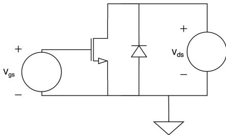
Figure 4.11: *NMOS with an external reverse diode*
