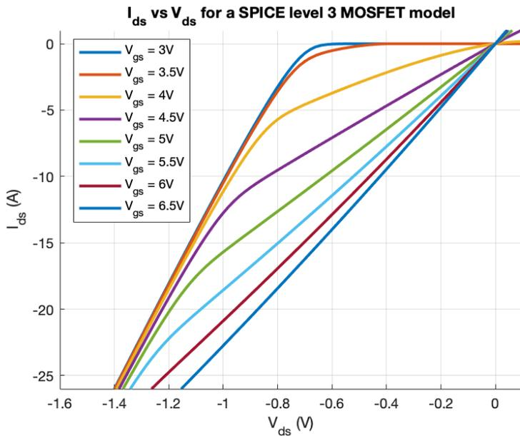
Figure 4.6:  $I_{ds}$  versus negative  $V_{ds}$  for different  $V_{gs}$  of a level 3 MOSFET model
