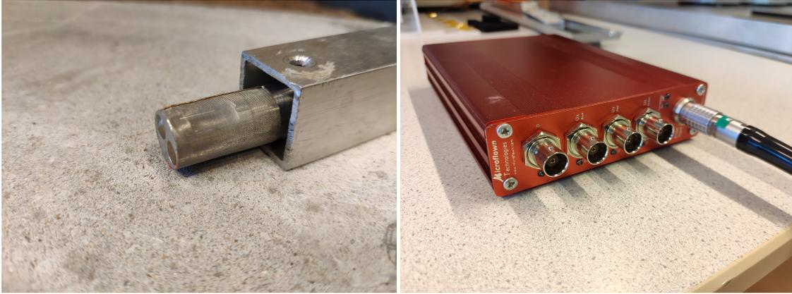
**Figure 3.4:** Particle velocity sensor setup - PU regular probe(left) and amplifier(right)
