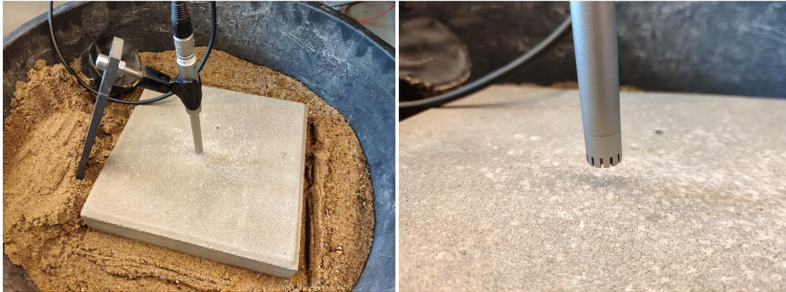
**Figure 3.2:** Microphone setup - overview of the microphone(left) and close up view(right)
