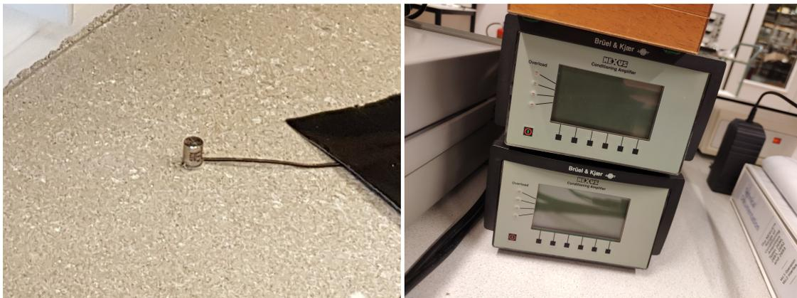
**Figure 3.3:** Accelerometer setup - type 4374 accelerometer(left) and charge amplifier(right)
