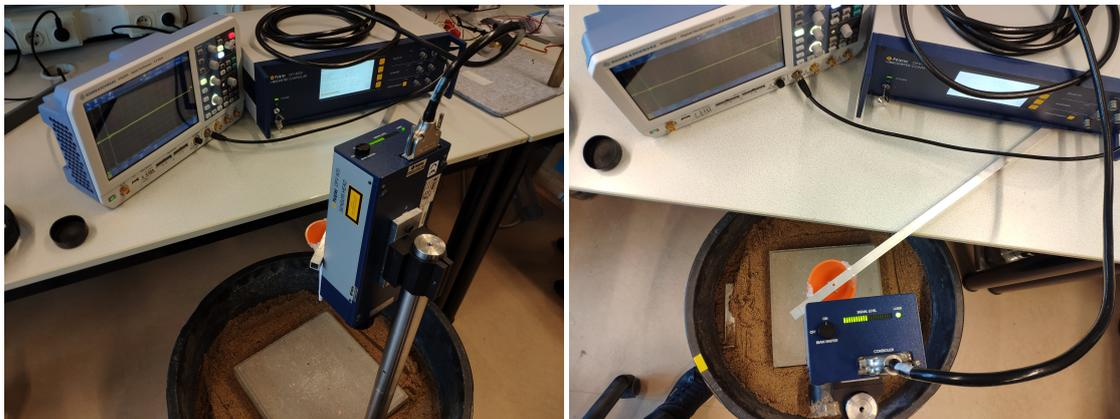
**Figure 3.1:** Laser vibrometer setup - overview of the setup(left) and top view(right)
