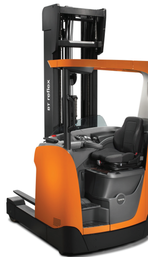
FIGURE 2.4: Reach truck. source: Toyota Material Handling
