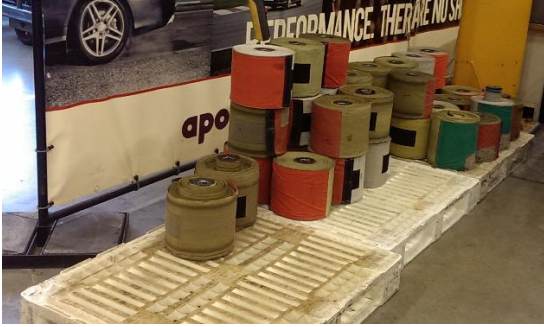
Figure 5c – Empty liners waiting to be inserted in Quadriplex
