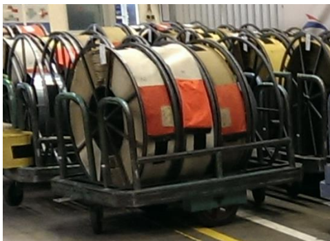
Figure 14c – Treads stored on HSP75 (reel) and LNHSP75 (liner) on CTREAD (cart) in LOLOS
