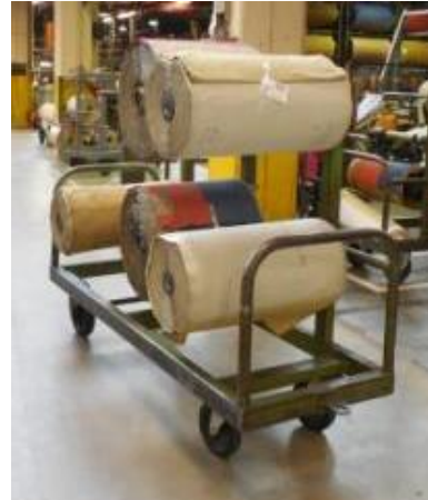
Figure 4(b) – loaded liner placed on cart after production
