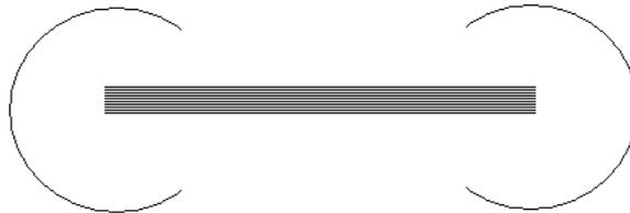
**Figure 3.10 Top-view of a microchannel with 10 parallel channels on the ‘pervaporation channels’ wafer**
