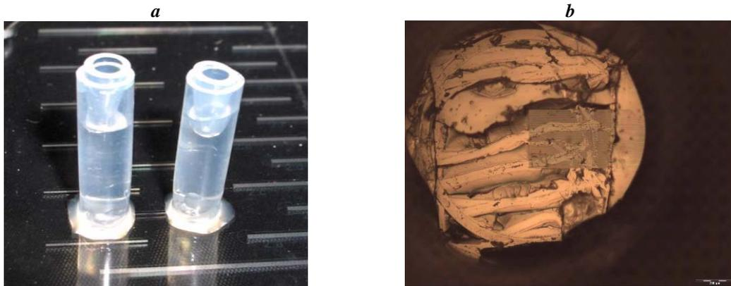
**Figure 3.31. a) Microchannels on a wafer, one microchannel has two reservoirs at the channel ends. b) top view of the bottom of a reservoir.**
