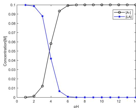
Figure 2.4. Acid-base equilibrium of lactic acid at a concentration of 0,1 M. Concentration of lactate ion [A<sup>-</sup>]. The concentration of lactic acid [LA] (adapted from[21])
