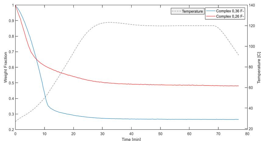
Figure 4.4 Weight losses of the complex coacervate at a composition of 0,36F- (blue line) and 0,26F- (red line) during the heating process as function of time. The temperature is plotted as function of time (dotted line).
