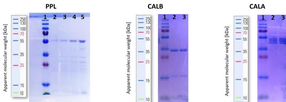
Figure 4.1. 12% SDS-page gel for PPL ( 1. Ladder, 2. 0,25 g/L, 3. 0,5 g/L, 4. 1 g/L , 5. 2g/L), CALB (1. Ladder, 2. 1 g/L, 3. 2 g/L) and CALA (1. Ladder, 2. 1 g/L, 3. 2 g/L)
