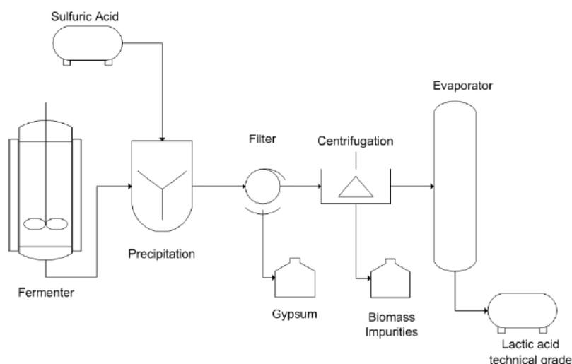
Figure 2.3. Layout of the conventional process for lactic acid recovery by precipitation[19]
