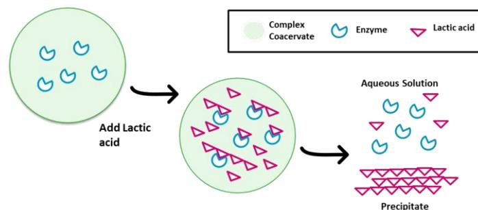
Figure 1.1. Proposed method to produce PLA from extracted LA
