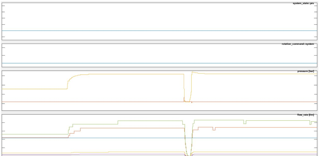
**Figure C.8:** A sudden drop in the pressure and flow rate of the cooling liquid.
