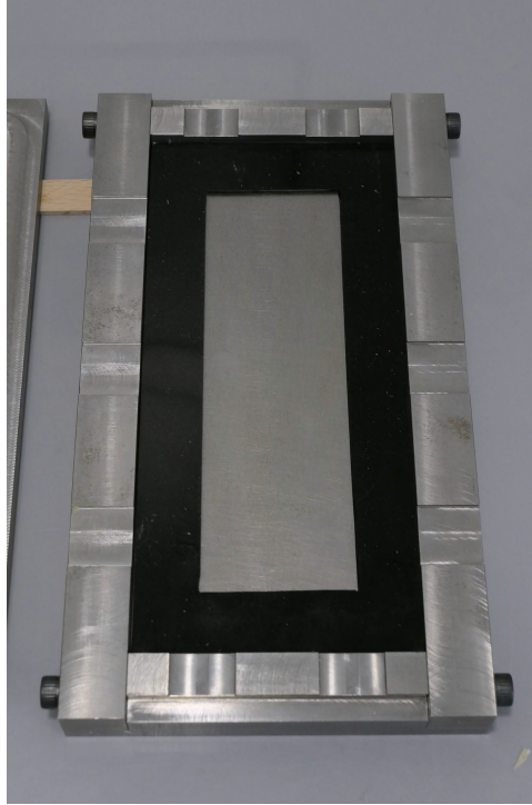
Figure 4.2: The opened bulk mould with the bottom plate, the four sides and a silicone frame. The top lid is not in the picture.
