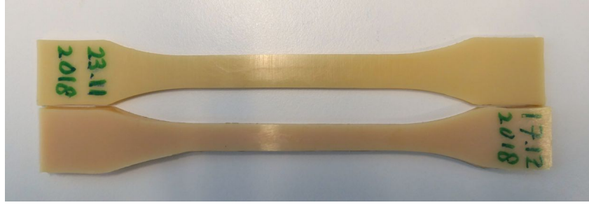
Figure 4.3: Two bulk dog bones. The top one is 2 mm thick and the bottom one is 4 mm thick. The discolouring of the bottom sample due to the exothermic reaction during curing can be clearly seen.
