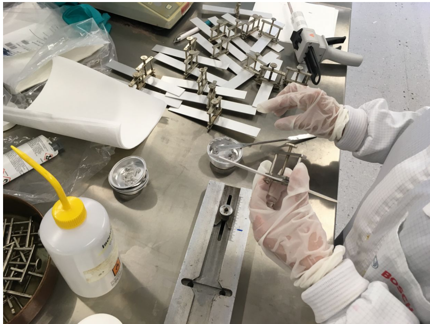
Figure 2.2: Gluing the specimens using the normal method. Below is the jig with the slider to control the overlap length. On top are glued samples and the glue dispenser.
