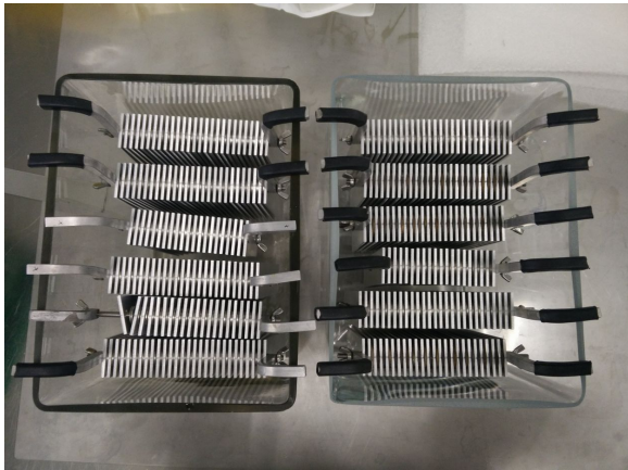
(a) Two batches with adherends hanging from the threaded rods.
