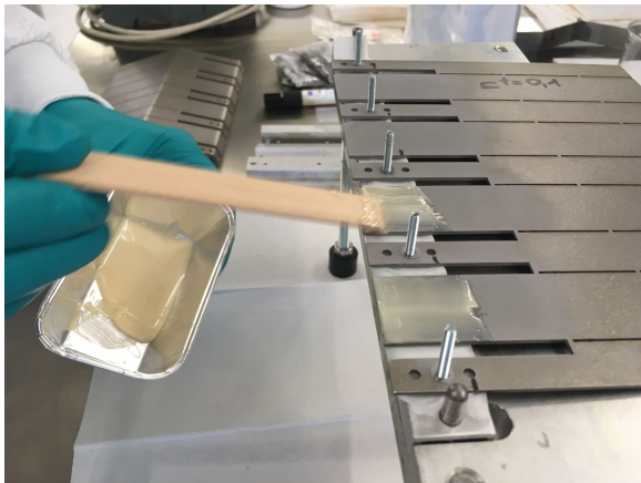
(e) Adhesive spread over the sample with a wooden spatula.
