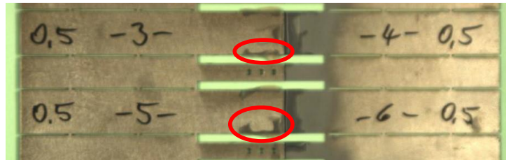
Figure 2.12: Adhesive on the outside of the samples, possibly pushing the adherends to each other.
