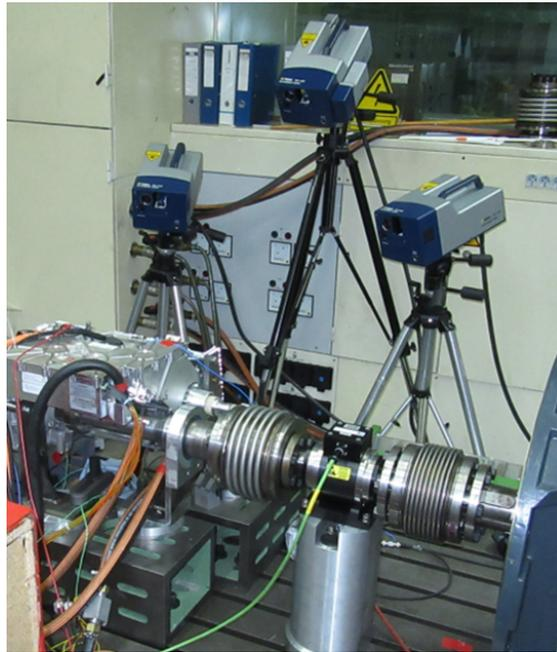
Figure 12: EMA setup with laser-vibrometers
