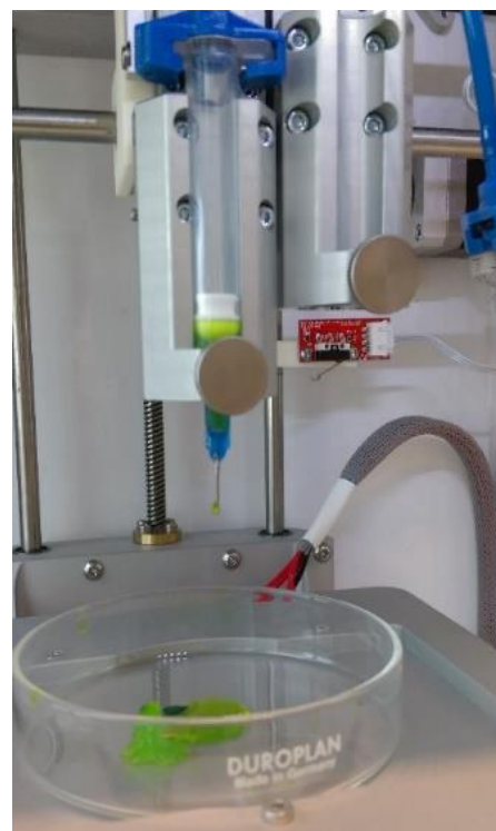
Figure 8. Printer set-up of the Cellink+ 3D printer. Ink was extruded through a 22G nozzle with a velocity of 10 mm/s and a pressure of 163 kPa and 181 kPa for respectively test 1 and 2.
