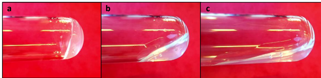
Figure 13. Mixed Dex 250 -βCD DS 6% #1 and Dex 250 -TA DS4%, from gel state towards fluid state at (a) t=0 min, (b) t=45 min and (c) t=60 min.
