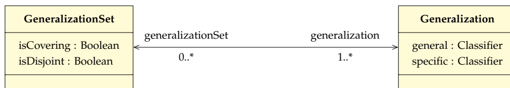
Figure 3.10: Simplified metamodel of UML Generalizations
