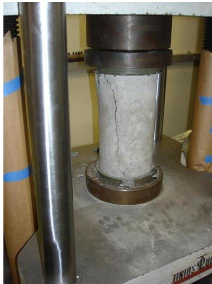
**Figure 2.12:** Example of compressive strength test on concrete
