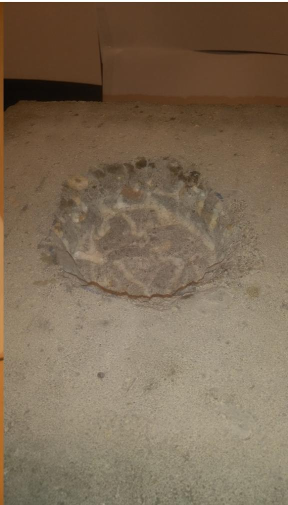
**Figure 3.13:** Concrete tile with a void
