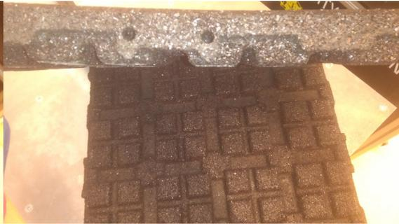
**Figure 3.15:** Downside of rubber tile
