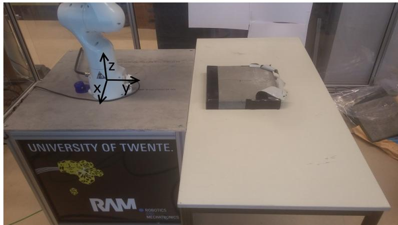
**Figure 3.16:** Placement of sample with axis
